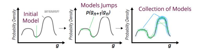
The jumps  $p(g_{n+1}|g_n)$  can be performed easily using the statistical behavior of memristors!
