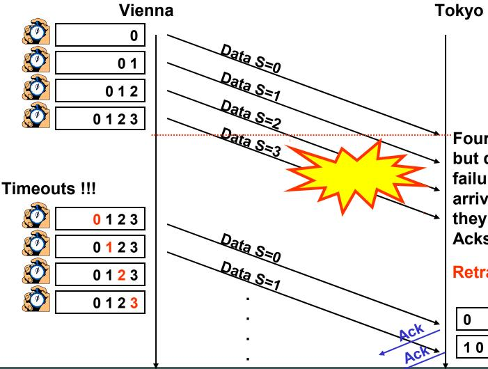
Four packets are sent, but due to a network failure none of them arrive (or equivalently they do arrive but the Acks are lost)
