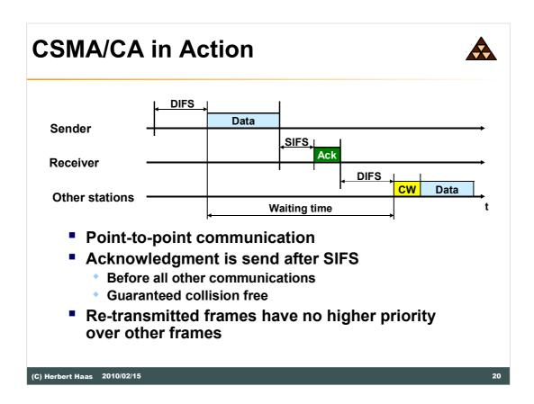
The picture above shows the DFWMAC with CSMA/CA method with a point-to-point communication. After the user data a acknowledgement is send. This acknowledgement is send after SIFS, so it will be transfer collision free and before all other communication. If a data packet need to be re-transmitted, the device need to wait DIFS and also using the normal backoff mechanism. This re-transmitted frames have no advantages compared with others.
