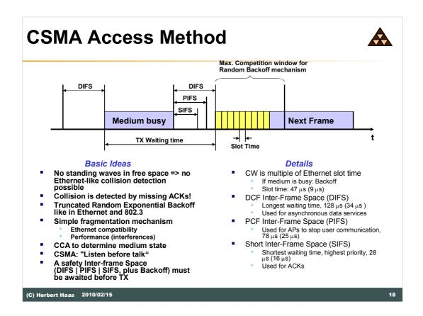
The picture above shows some important parameters which are necessary before a device can access on a medium. DIFS, PIFS and SIFS control the priority before a device can have access. A medium can be full or busy, the current status will be detect with the help of the CCA signal.
