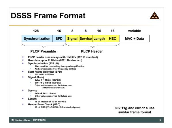
The DSSS frame format shown here is used by 802.11b but the frame format is also valid with 802.11g and 802.11a except that the values for the fields are different.
