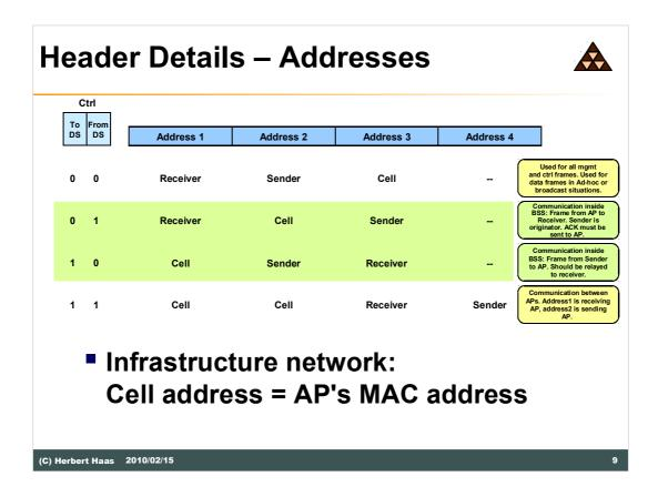
Four addresses are used in bridging mode but bridging is a very proprietary feature with lots of additional undocumented tricks.
