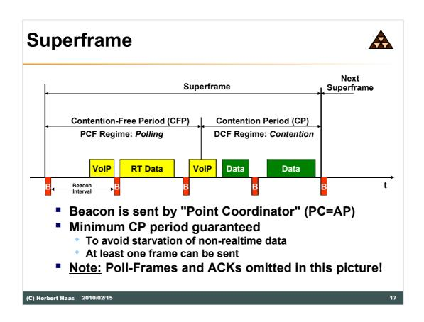
Typically the Point Coordinator (PC) is integrated in the AP but this is not required. In order to give an idea of the basic principle of the superframe, the CFP and the CP, many details have been omitted. The details of both periods are explained in the following slides.
