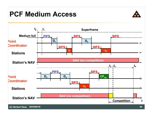
The picture above shows the schematic view of the DFWMAC-PCF method. Remember the data transfer take place by the point coordinator. All data will be send or received from or by the point coordinator.  $D_n$  and  $U_n$  are data/user-data from or to the point coordinator.
