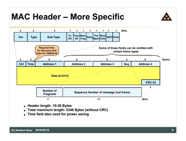
2312 bytes max frame length without encryption etc.
