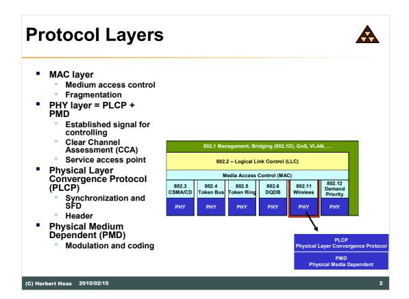
The 802.11 standard only describes the physical and the MAC layer. The physical layer is split into the PLCP and the PMD protocol. The Medium Access Control takes-over the layer 2 functions.
