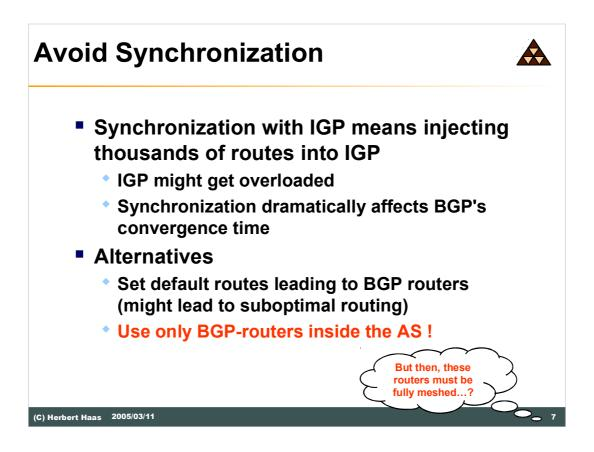
Synchronization is an old idea and leads to unwanted effects. First of all, most IGPs are not designed to carry a huge number of routes as needed in the Internet. Thus IGPs might get overloaded when ten thousands of external routes should be propagated in addition to the interior routes.
