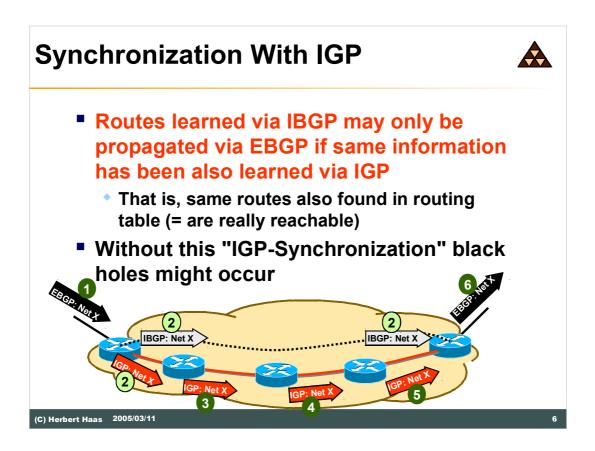
When a BGP router learns about an exterior network via an IBGP session, this router does not enter this route into its routing table nor propagates this route via EBGP because the IGP-transit routers might not be aware about this route and therefore convergence has not been occurred yet. The BGP router should propagate the learned route until this route has been entered into its routing table by IGP.
