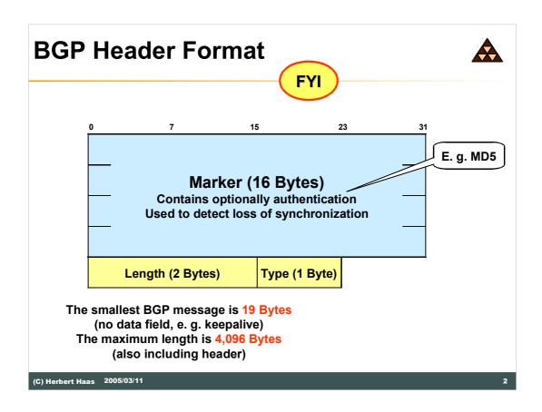
This is the basic BGP header format. This and the following slides marked with a "FYI" at the upper-left of the slide are only given "for yout interest". It is usually not necessary to know this details by heart—unless you plan to go deeper in BGP.
