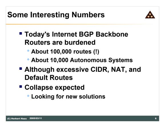
Internet routers do a hard job. The number of networks is increasing exponentially since the early 1990s and the only way to overcome routing table exhaustion is to apply excessive supernetting (CIDR), NAT, and default routing. In 2001 about 100,000 routes have been counted in typical BGP Internet router. Moreover, 10,000 ASs have been registrated.
