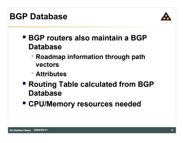
The designers of the BGP protocol have succeeded in creating a highly scalable routing protocol, which can forward reachability information between Autonomous Systems, also known as Routing Domains. They had to consider an environment with an enormous amount of reachable networks and complex routing policies driven by commercial rather than technical considerations.
