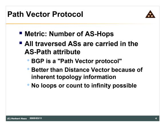
Each BGP update consists of one or more IP subnets and a set of attributes attached to them. The intrinsic metric is the number of AS hops. Note that this metric is given implicitly by a AS path attribute, which is a vector of all ASs traversed.
