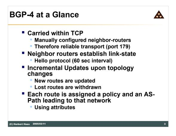
A router which has received reachability information from a BGP peer, must be sure that the peer router is still there. Otherwise traffic could be routed towards a next-hop router that is no longer available, causing the IP packets to be lost in a black hole.
