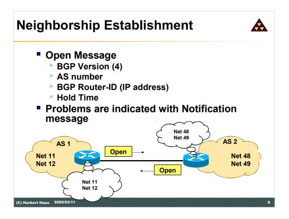
The BGP protocol is carried in a TCP session, which must be opened from one router to the other. In order to do so, the router attempting to open the session must be configured to know to which IP address to direct its attempts.
