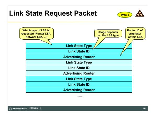
Note that the Link State Request Packet uniquely identifies the LSA by Type, ID, and advertising router fields of its header. It does not include the sequence number, checksum, and age, because the requestor is not interested in a specific instance of the LSA but in the most recent instance.
