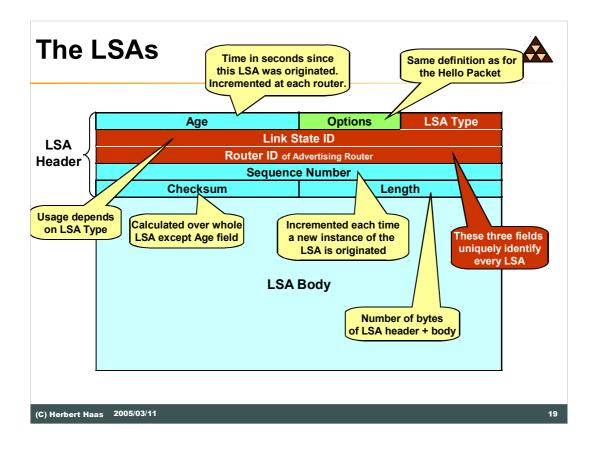
All LSAs have the LSA header at the beginning. This LSA header is also used in Database Description and Link State Acknowledgement packets.
