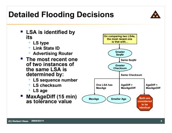
Each LSA carries also a 16 bit age value, which is set to zero when originated and increased by every router during flooding. LSAs are also aged as they are held in each router's database. If sequence numbers are the same, the router compares the ages the younger the better but only if the age difference between the recently received LSA is greater than MaxAgeDiff; otherwise both LSAs are considered to be identical.
