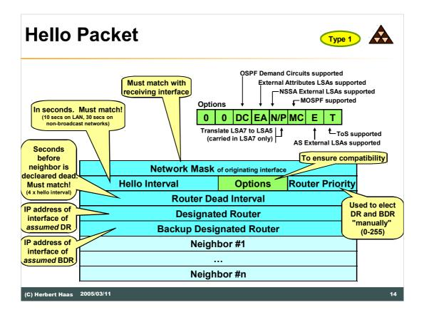
The network mask must match the mask on the receiving interface, ensuring that they share a segment and network.
