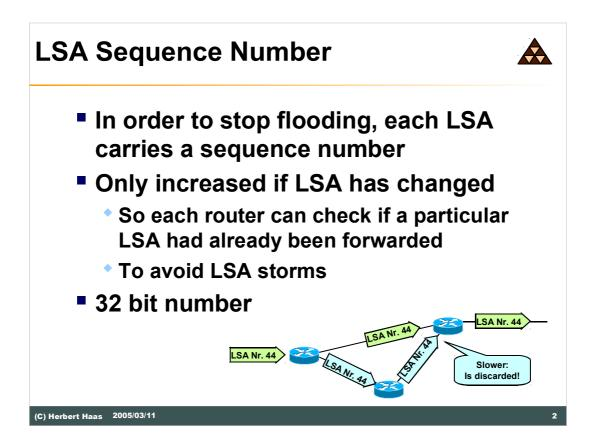
When reaching the end of the 32 bit sequence number the associated router will wait for an hour so that this LSA ages out in each link state database. Then the router resets the sequence number (lowest negative number i. e. MSB=1, 80000001) and continues to flood this LSA.
