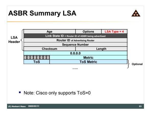
A ASBR Summary LSA is originated by an ABR and advertises ASBRs external to an area.
