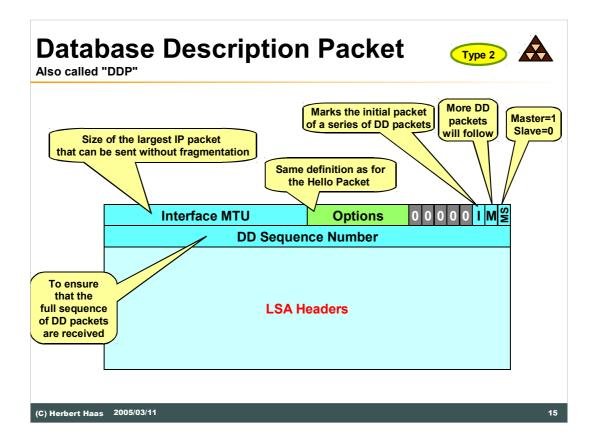
The DD sequence number is set by the master to some unique value in the first DD packet. This number will be incremented in subsequent packets.
