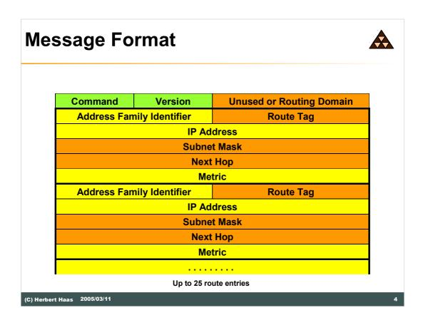
RIPv2 utilizes the unused fields of the RIPv1 message-format. New fields are the "routing tag", "subnet mask" and the "next hop".
