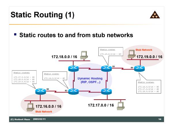
In the picture above we see a good example of static routes. Every router in the stub networks is configured manually, because there is only one way the packet can go. Most of the time this entries are set to permanent, so the routes need not be configured again when the interface goes down.
