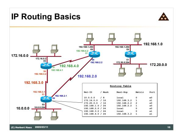
In the picture above there is small network, and a good example of a routing table. For example a host in network 10 want to send a packet to a user in network 192.168.1.
