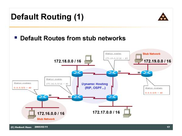
In this example you see the work of default routing. Every packet a router of a stub network receives will be forward to the next router, doesn't matter what destination address.
