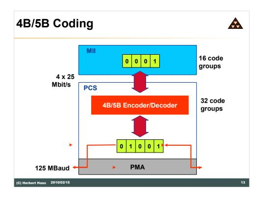
The diagram above shows the basic principle of the 4B5B block coding principle, which is used by 802.3u and also by FDDI. The basic idea is to transform any arbitrary 4 bit word into a (relatively) balanced 5 bit word. This is done by a fast table lookup.
