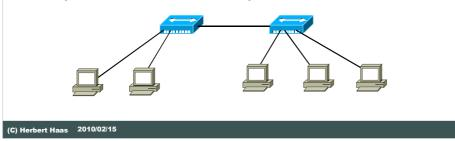
Later, Ethernet devices supporting structured cabling were created in order to reuse the voice-grade twisted-pair cables already installed in buildings. 10BaseT had been specified to support Cat3 cables (voice grade) or better, for example Cat4 (and today Cat5, Cat6, and Cat7).
