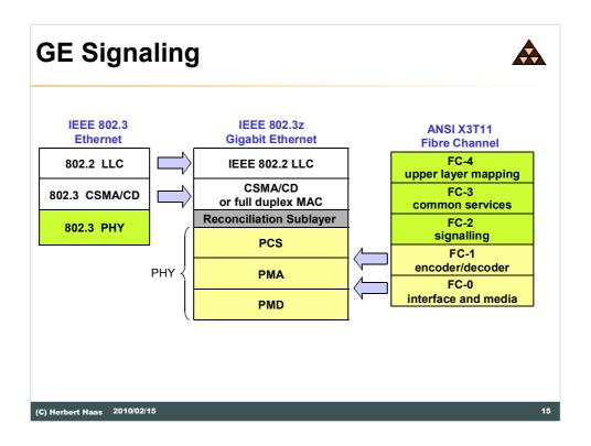
Gigabit Ethernet layers have been defined by adaptation of the LLC and MAC layers of classical Ethernet and the physical layers of the ANSI Fiber Channel technology. A so-called reconciliation layer is used in between for seamless interoperation. The physical layer of the Fiber Channel technology uses 8B10B block coding.
