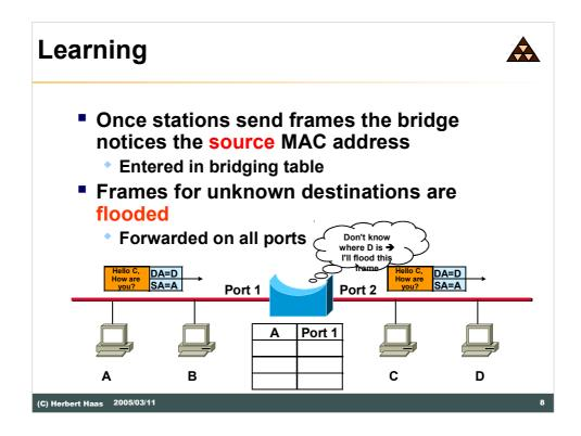
Assume we have a bridge with only two ports, each attached at one Ethernet segment. Assume the left station "A" sends one frame to "D" on the right side. Obviously the bridge learns the location of A but has no idea where D is. Thus the MAC address of A is entered in the bridging table and also the port number "1", on which A is reachable. Since the location of D is unknown, the bridge bridge floods this frame over all ports, in our case only to port two (as there are no other ports).
