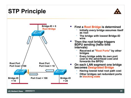
We give only a basic explanation here of how the STP works. First a **Root Bridge** is determined by choosing the bridge with the **lowest** Bridge-ID. This is simply done by sending BDUs containing the presumed Root Bridge. At first each bridge assumes to be the Root Bridge itself. After any bridge has sent his "opinion" the root bridge is determined.
