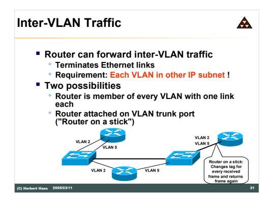
Now we admit the wholly truth: of course it is possible to communicate between different VLANs—using a router! A router terminates layer 2 and is not interested in VLAN constraints. Of course this requires that each VLAN uses another subnet IP address since the router needs to make a routing decision.
