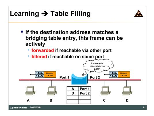
Now assume D replies to the message which has been received from A. The bridge knows already the port number over which A can be reached and forwards the frame accordingly. If A would be located on the same port as D then this frame would be filtered.
