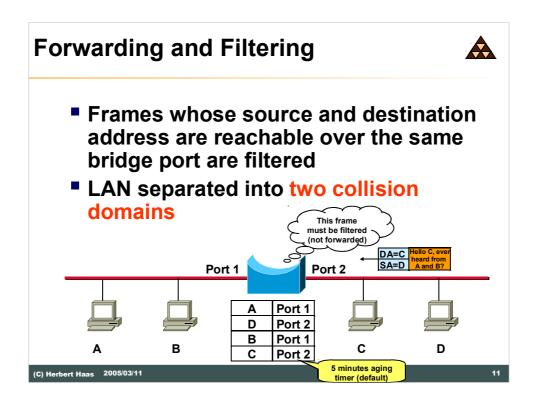
Since only frames are forwarded to other ports whose destination is really located there, the LAN is separated into as many collision domains as ports are available (and attached to a LAN segment).
