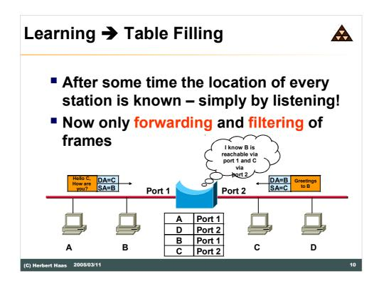
After some traffic observing time, the bridging table contains all host locations (addresses and port numbers). At this time the bridge enters the forwarding and filtering mode.
