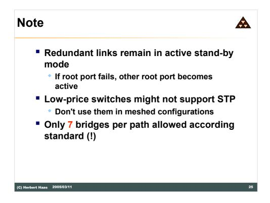
Still it is reasonable to establish parallel paths in a switched network in order to utilize this redundancy in an event of failure. The STP automatically activates redundant paths if the active path is broken. Note that BPDUs are always sent or received on blocking ports.
