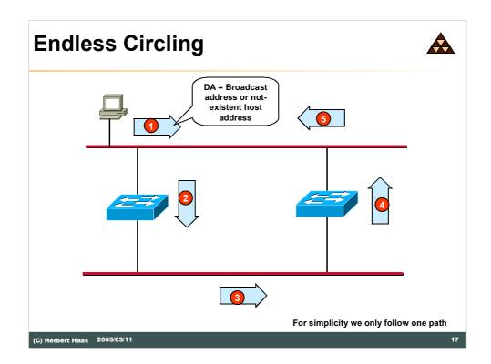
The picture above illustrates the endless circling phenomena. Assume a network with parallel paths between two LAN segments, realized by two bridges. Any frame with a broadcast destination address would be forwarded by both bridges to the other segment and back and forth and so on.
