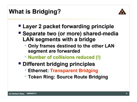
Bridges forward layer 2 packets (frames) according to their destination address. Hereby, those frames are filtered whose destination is not reachable on another port of the bridge. This filtering capability significantly enhances the total performance of a LAN as it is divided into multiple segments—multiple broadcast domains: The number of collisions is reduced!
