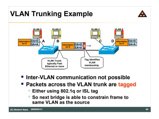
By using VLAN tagging the "next" bridge knows whether the source address is also member of the same VLAN.
