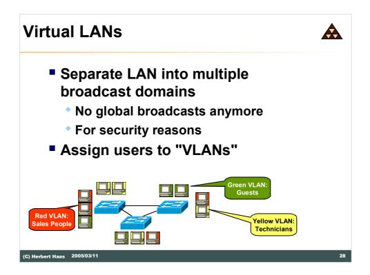
Since most organizations consist of multiple "working groups" it is reasonable to confine their produced traffic somhow. This is achieved using Virtual LANs (VLANs). Switches configured for VLANing are consist logically of multiple virtual switches inside.
