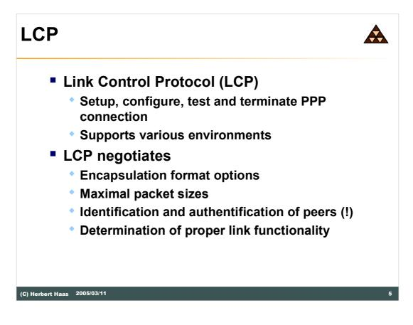
In order to be sufficiently versatile to be portable to a wide variety of environments, PPP provides a Link Control Protocol (LCP). The LCP is used to automatically agree upon the encapsulation format options, handle varying limits on sizes of packets, authenticate the identity of its peer on the link, determine when a link is functioning properly and when it is defunct, detect a looped-back link and other common misconfiguration errors, and terminate the link.
