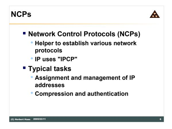
Point-to-Point links tend to exacerbate many problems with the current family of network protocols. For instance, assignment and management of IP addresses, which is a problem even in LAN environments, is especially difficult over circuit-switched point-to-point links (such as dial-up modem servers). These problems are handled by a family of Network Control Protocols (NCPs), which each manage the specific needs required by their respective network-layer protocols.
