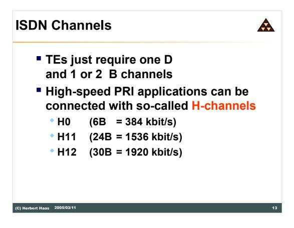
H channels are bundles of B channels to obtain a higher data rate.
