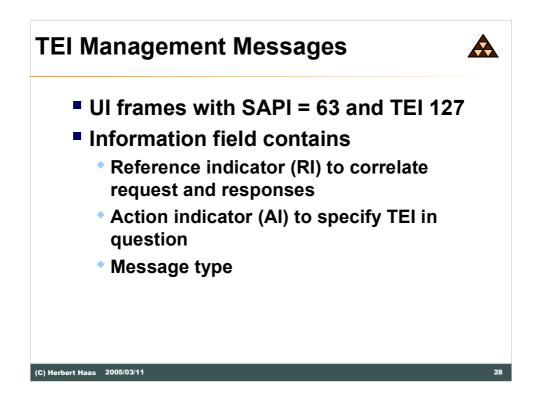
Also management messages are identifed by a special SAPI (63), combined with a TEI of 127, which addresses **all** TEs (broadcast). These management messages are used to assign TEIs to the TEs.
