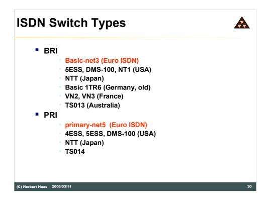
When configuring the ISDN devices it is very important to know about the switch (LE) type because there are many flavors.
