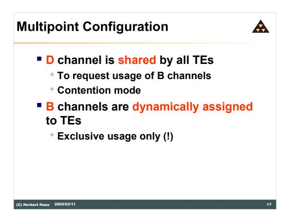
The multipoint configuration is typically used for private users. Here the D channel is shared by up to 8 TEs. The D channel is used similarly as an Ethernet bus medium—contention takes place! The winner gets a B channel for communication. This B channel is dynamically assigned but immediately released when the call is terminated.
