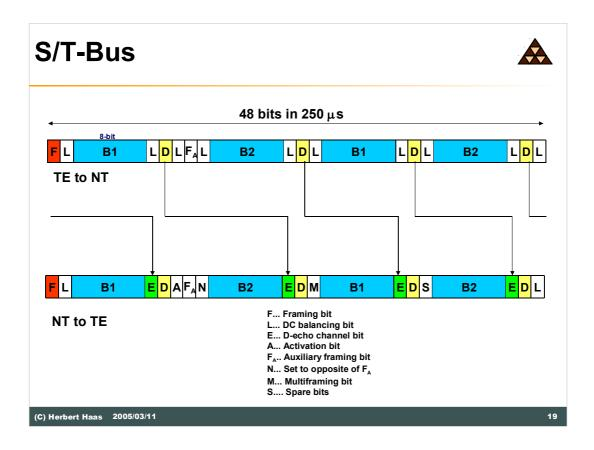
F (+) followed by L(-) marks start of frame. To prevent F in the bit stream, code violations are used (normally alternate pulses (+, -) used for zeroes)
