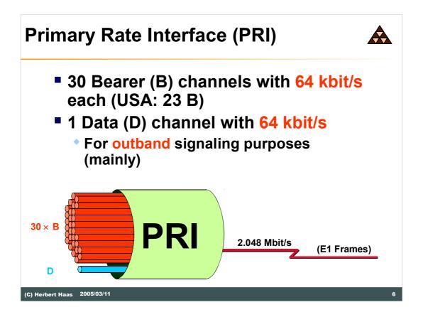
The PRI also contains B and D channels, but now there are 30 B channels and also the D channel has the same bandwidth of 64 kbit/s. These 31 channels plus an additional synchronization channel result in a total data rate of 2,048 Mbit/s, which is transported over a so-called E1 frame.
