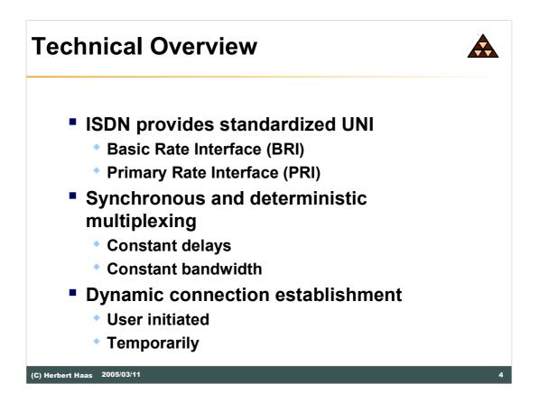
ISDN specifies only a User to Network Interface (**UNI**)—quite similar than X.25 and Frame Relay. But the main difference is that ISDN relies on deterministic, synchronized multiplexing.
