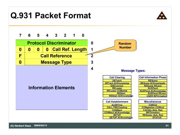
The Q.931 packet format is given in the picture above only to provide a consistent ISDN overview here. It is not necessary to memorize this structure in detail.
