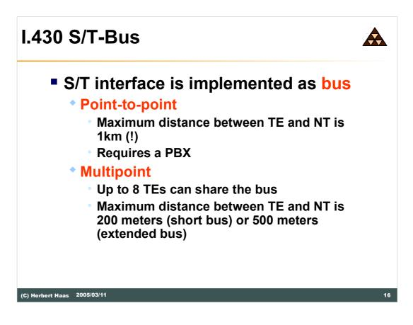
An ISDN interface can be configured either in multipoint mode or in point-topoint mode.
