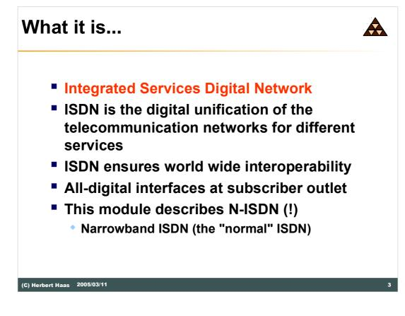
N-ISDN means **Narrowband-ISDN**, but you can also think of "Normal-ISDN". The planning of ISDN began already in 1976, but real-world applications became available only with the mid-80's. Also Frame-Relay is regarded as part of the ISDN family, because it can be transported upon the physical layer of ISDN, which we will discuss soon.
