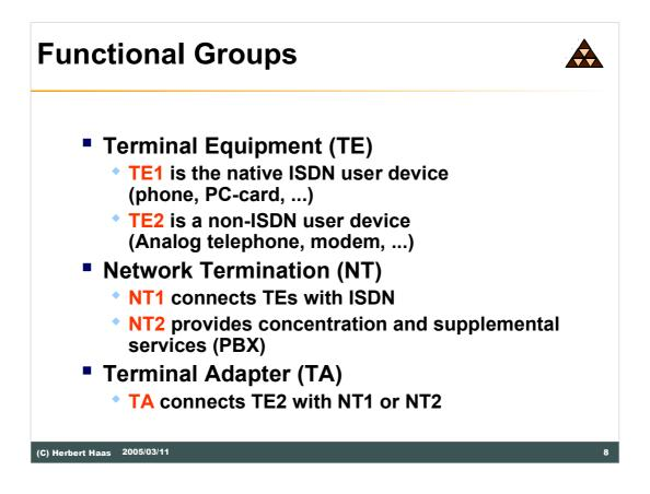
Several "functional groups" have been specified to differentiate technical capabilities. An end device is called a "Terminal Equipment" (TE).
