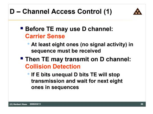
In multipoint mode the S7T bus is used in contention mode similar to Ethernet. Before a TE may use the D channel it must listen whether some TE is sending —"carrier sense" is performed. Here at least eight "1" must be received in sequence. Since the inverse AMI coding is used this means that nobody is currently sending.
