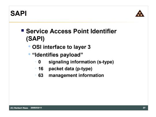
Additionally a Service Access Point Identifier (SAPI) is needed to identify the content of this LAPD frame. Each SAPI number identifies a layer 3 service. For example Q.931 services might be addressed or the SAPI might also indicate that the LAPD payload is a X.25 data frame.
