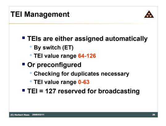
Note that the TEI is not used for primary rate interfaces (PRI) because PRI do not support multipoint connections. Here the TEI is always set to zero.
