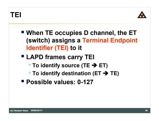
A switch (LE) would not really know which TE is currently actice and has grabbed the D channel. Therefore a Terminal Endpoint Identifier (TEI) is assigned to the TEs. The LAPD frames carry the TEI which can be compared to an Ethernet MAC address while the telephone number is similar to an IP address in this context.
