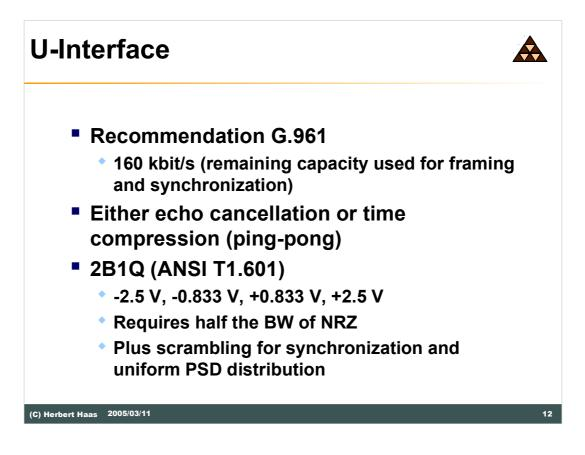
The U-interface is defined in CCITT "Recommendation G.961" and specifies a 160 kbit/s transmission method over two wires. Bidirectional communication is provided either by echo cancellation or "ping-pong" transmission, i. e. alternating sending and receiving of both sides within short time periods.
