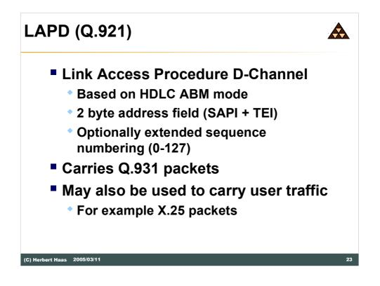
Note that the D channel is empty in most of the time because its only needed when establishing or closing a connection. Because of this, many providers allow to send user data over the D channel, using for example X.25. Of course this is no free service, because the provider network has to transport this data, so users have to pay for it.
