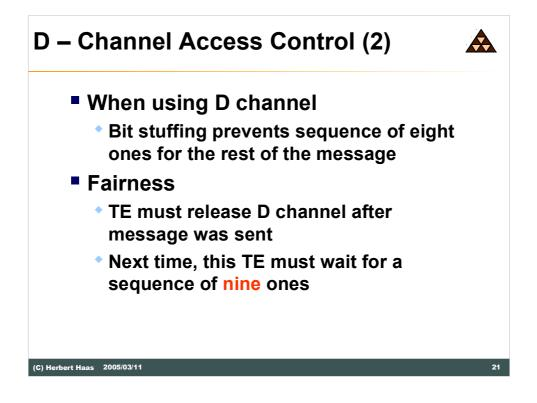
Of course measures must be implemented to avoid eight ones during sending another TE might assume that the S/T bus is empty! Thus bit stuffing is performed in such cases (inserting a zero).
