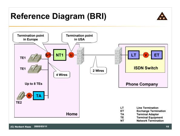
A TE2 is for example a plain old telephone (POT) or an analog modem. The R interface is typically a EIA/TIA-232-C, V.24, or V.35.
