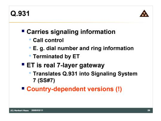
Q.931 is a signaling protocol used by N-ISDN and also (slightly enhanced) by B-ISDN. Using Q.931 the dial number is forwarded to the Telco switch, which terminates the D channels and puts all signaling information on top of another signaling protocol. Typically SS#7 is used in most Telco networks.
