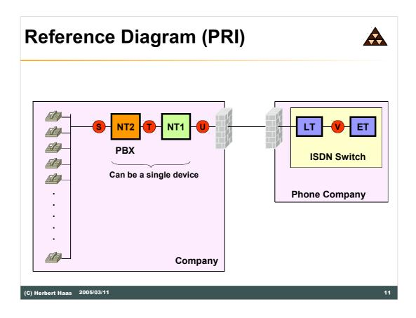
The picture above shows the principle of a PRI installation, using a PBX (NT2) which terminates all local telephones. Note that these telephones are not necessarily ISDN compliant telephones. Rather vendor proprietary technologies are used here.
