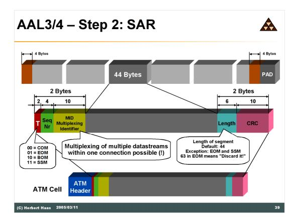
The sequence number enumeratess each 44 byte segment of the CS frame (modulo 16). The Multiplexing Identifier (MID) allows to multiplex up to 210 different connection-oriented AAL 3/4 connections. For connectionless packets, the MID field can be used as unique identifier associated with each user, in order to multiplex many users over one ATM pipe.
