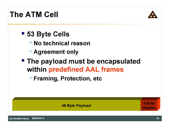
USA proposed a cell size of 64 bytes while the Europeans suggested 32 bytes. At the end they met in the middle at 53 bytes.
