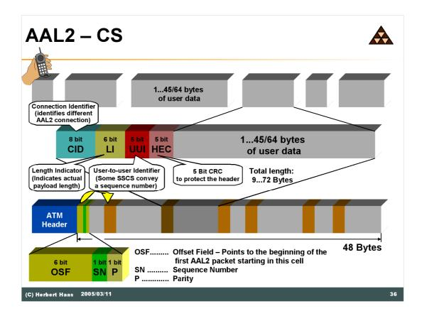
The slide above shows the most important tasks of the Common Part Convergence Sublayer (CPCS). Basically, CPCS-packets consist of a one-byte header and up to 45 bytes user data (typically compressed voice or video). Even longer payloads are supported if an appropriate SSCS is used additionally (I.366.1).
