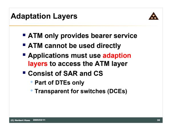
The ATM adaption layers translate between the specific worlds of higher layer protocols such as IP, X.25, or PCM-Voice and the cell-nature of the ATM layer itself. Using specific adaptation layers, nearly every application can be transported over ATM. This capability emphasizes again the B-ISDN idea that has been realized.
