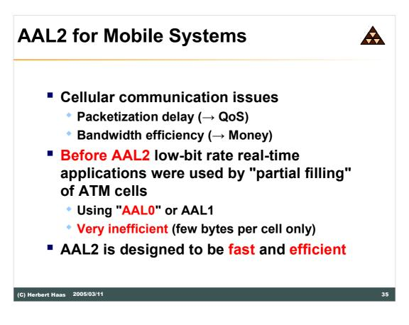
AAL0 simply means using ATM without any adaptation layer. The AAL2 CPCS allows variable packet length between 1 byte to 45 bytes, so the packetization delay can be kept very small, if needed. On the other hand, bandwidth efficiency is achieved by multiplexing several AAL2 connections within one ATM (VPI/VCI) pipe.
