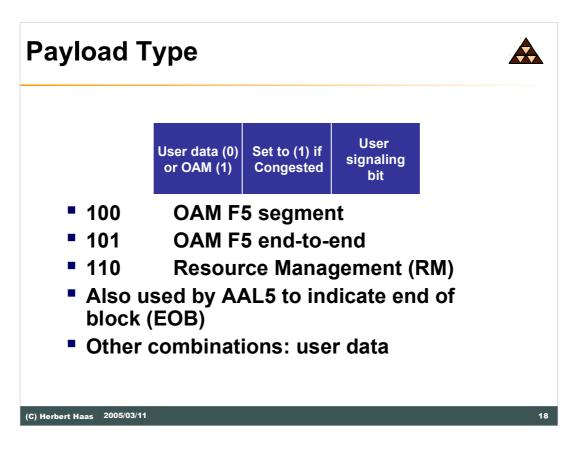
"Flow 5" (F5) is identical to a VC, F4 is the VP flow, F3 is a SONET/SDH Path, F2 is a SONET Line (SDH Mux-section), F1 is a SONET section (SDH regenerator section).
