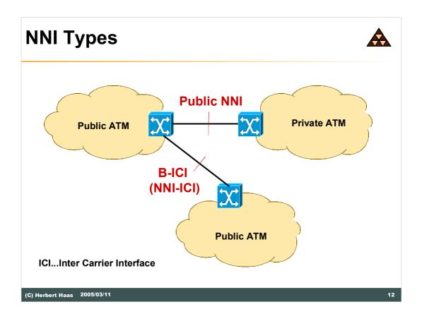
NNI-ISSI (Public NNI) ISSI = Inter Switch System Interface Used to connect two switches of one public service provider
