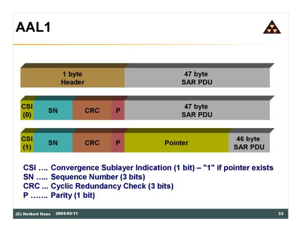
The CSI values in cells 1, 3, 5, and 7 are interpreted as a 4 bit timing value in order to measure timing differences between network's reference clock and transmitter clock. The 3 bit CRC only protects the 4 bit CSI+SN field. The parity bit is set such that the parity of the 8 header bits is even.
