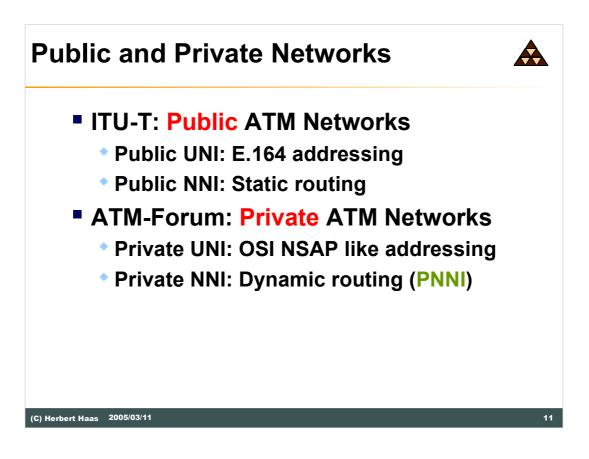
Note that both public and private networks cover SVCs but in order to establish SVCs we need routing tables. The routing tables can be created automatically in private ATM networks using the ATM routing protocol PNNI (Private-NNI). In public networks the routing tables are managed manually.
