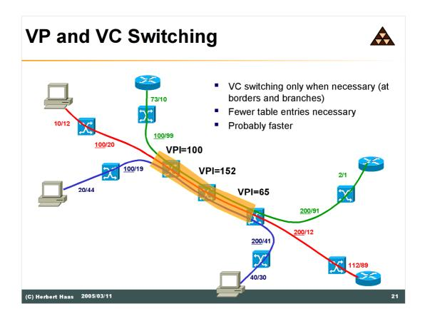
If one customer asks for another 100 virtual circuits, the provider does not need to add 100 additional entries in every switching table—as he must do with Frame Relay for example—because one VPI represents a number of VCIs and inside the network VPI switching is performed.
