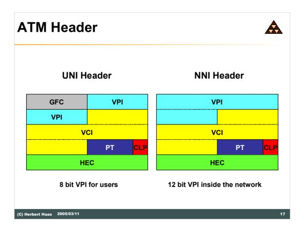
The Generic Flow Control (GFC) field is only used on the UNI but not transported into the network. The GFC is not used today as there are better methods available (special flow-control cells).
