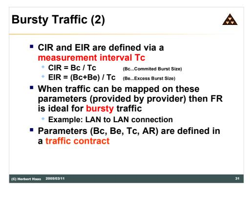
The CIR and the EIR are defined via a measurement time interval Tc, which is set to 1 second in most cases. The committed burst size Bc defines the amount of bits per Tc with guaranteed delivery. The Excess Burst Size Be specifies the maximum allowed oversubscription of bits per Tc, for which the delivery will not be guaranteed.
