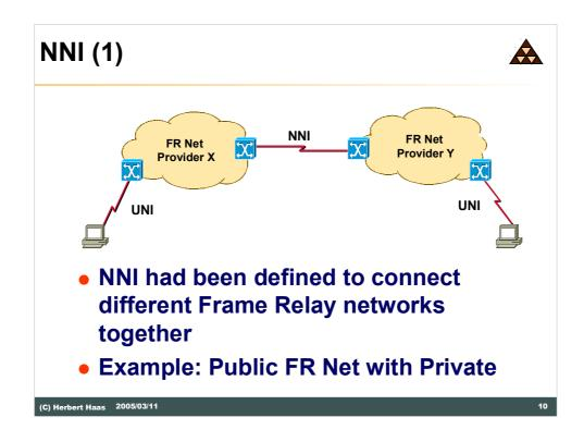
Due to the fact that the Frame-relay standards to not cover the Frame-relay cloud itself a Frame-relay Network to Network Interface (NNI) was standardized to allow the connection of different Frame-relay networks under the use of different vendor equipment. The NNI interface standardizes the FR-DCE to FR-DCE communication e.g. in the case of connection a private Frame-relay network to a public Frame-relay network.
