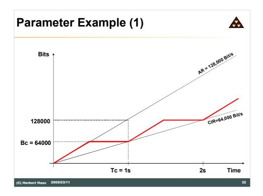
In this example the measurement time interval Tc is set to 1second, the Bc to 64000 bits and the physical access rate is 128 Kbit/s. The red line indicates the actual traffic pattern used on this connection. In this scenario the traffic characteristic remains within the CIR of 64 Kbit/s.
