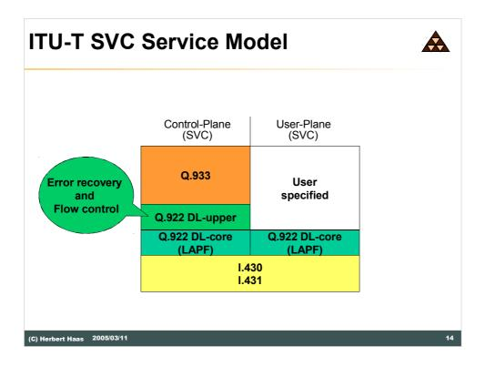
But Frame Relay can also support SVC services. In this case we don't use Annex A but rather plain "Q.933". Furthermore SVC mode requires a reliable Q.922 connection to the DCE, which is handled by the so-called "Q.922 DLupper". The Frame Relay layer itself is the Q.022 DL-core layer, which must be always existent.
