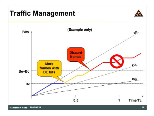
This example shows us what might happen if more traffic is injected than the Frame-relay traffic parameters allow. Obviously the behavior in real life is completely up to the traffic contract negotiated and might be different from our scenario.
