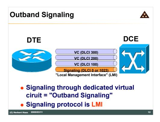
The Local Management Interface (LMI) was developed to inform the Framerelay users about the condition of the Frame-relay network itself.
