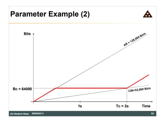
In this scenario a measurement interval Tc of 2 seconds is chosen. The committed burst size Bc is 64000 bits, so the CIR according to the formula CIR = Bc / Tc will be 32 Kbit/s. The actual traffic pattern indicated by the red line remains again within the borders of the CIR.
