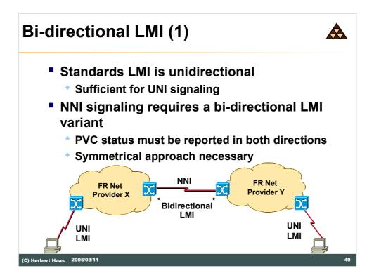
Common LMI is unidirectional and can only be used for UNI interfaces.
