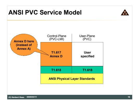
In this slide the corresponding standards of the ANSI committee for Framerelay PVC service can be seen. The ANSI standard T1.618 describes the basic Frame-relay frame with DLCI, BECN, FECN, etc. and it corresponds to the Q922 core standard from the ITU-T.
