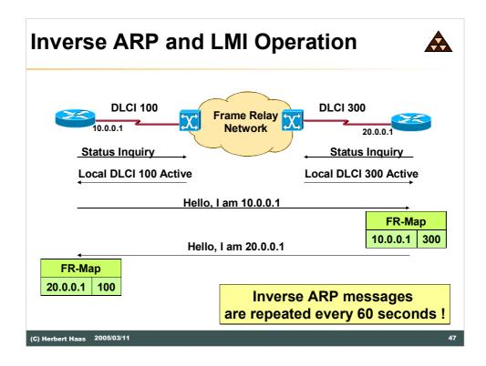
In this scenario the function and the interaction of the LMI and the Inverse ARP protocol is shown.
