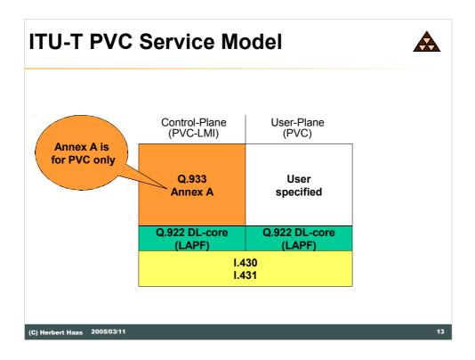
Every protocol that employs outband signaling has a vertically divided layer architecture. Here the left part (in the slide above) correspond to the layers used for outband signaling while the layer stack on the right hand handles data packet delivery through virtual circuits. Additionally, the outband path is called the "Control Plane" and the data-VC path is called the "User Plane". Take it as it is.
