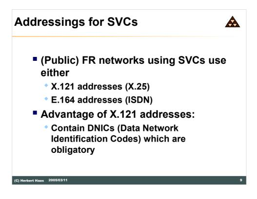
Although only a few service providers offer SVC Frame Relay service it is still possible and part of the standard. In order to establish an SVC a DTE must know a globally unique host address of the destination. Typically, the X.121 or E.164 address plans are also utilized for Frame Relay. Don't confuse X.121 and E.164 addresses with the priviously mentioned global addresses.
