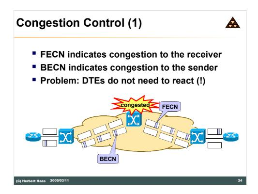
The Frame-relay network is able to indicate congestion situations to its users by the help of the BECN and FECN bit located in the Frame-relay header.
