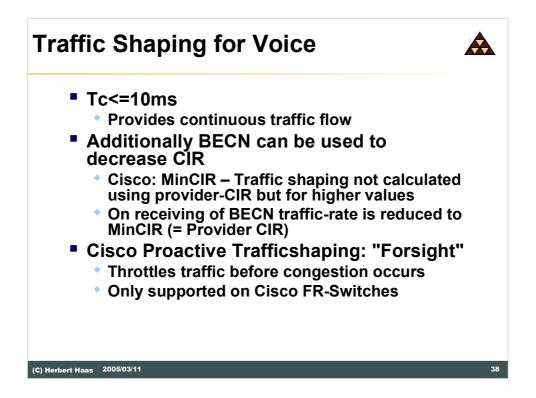
Traffic shaping for voice is much more delay and jitter sensitive than for data. To accomplish to the needs of voice Tc is set from 125 milliseconds used for data to a value below 10 milliseconds to generate a continuous traffic flow with minimum jitter. These needs to be done obviously in combination with the configuration of smaller datagram sizes between 50 to 100 bytes.
