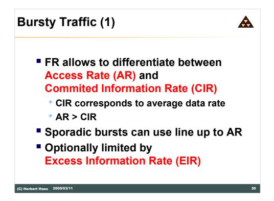
As already discussed before the main parameters that determine the transport capacity of a Frame-relay connection are the physical AR, the CIR and the Excess Information Rate (EIR).
