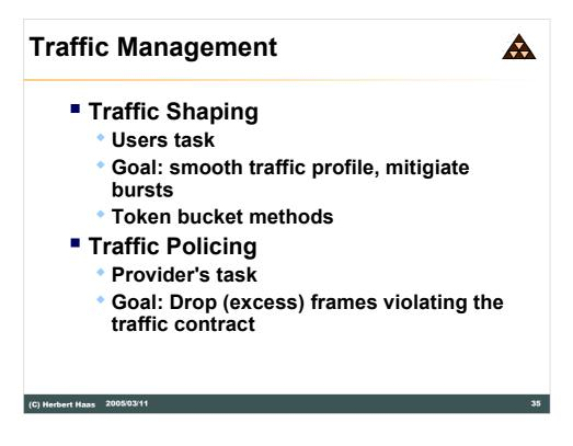
Traffic shaping according to the negotiated parameters is in the responsibility of the end users. End users traffic that is outside the traffic contract will be discarded by the first Frame-relay switch in the providers network.
