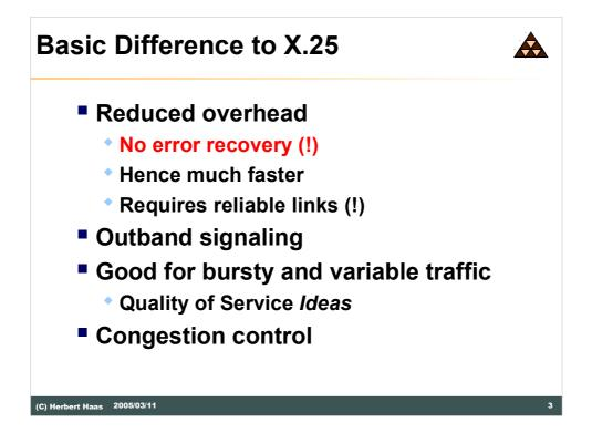
The most important difference to X.25 is the lack of error recovery and flow control. Note that X.25 performs error recovery and flow control on each link (other than TCP for example). Obviously this extreme reliable service suffers on delays. But Frame Relay is an ISDN application—and ISDN provides reliable physical links, so why use ARQ techniques on lower layers at all?
