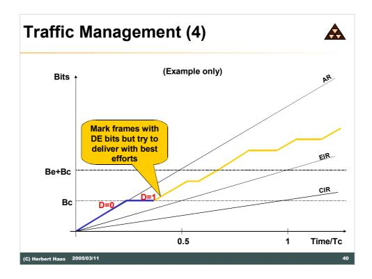
This is the typical service provider behavior. Typically, a customer just pays for the CIR and the rest of the bandwidth – up to the access rate – is free. However, there is no gurantee that every excess packets is delivered to the receiver.
