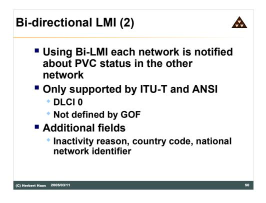
When bidirectional LMI is used every network gets the PVC status information of the opposite side. Bidirectional LMI is only supported by the ANSI and the ITU-T standard and uses the same DLCI number that is used for unidirectional LMI.
