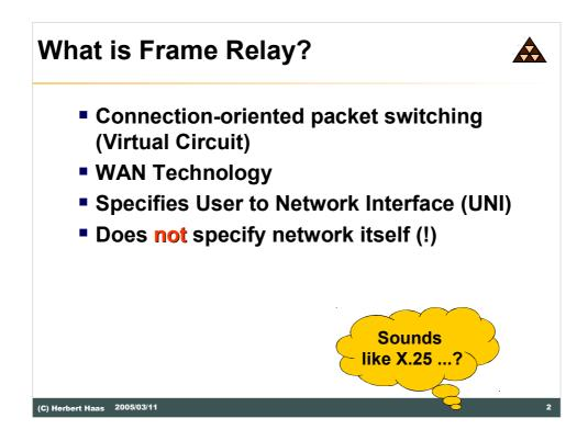
Frame-relay is a technolology that appeared in the beginning of the 1990's and was developed to replace X25 WAN technology.
