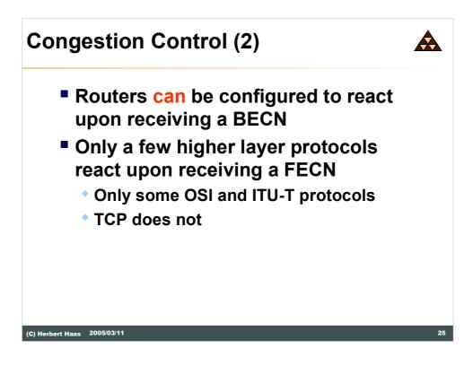
So the sender will receive its packets with the BECN bit set while the receiver receives packets with the FECN bit set. Now its completely up to the sender to reduce the amount of traffic it injects (traffic shaping configurable by software).
