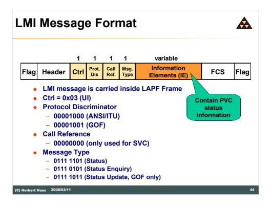
The LMI messages are packed in standard Frame-relay frames and are transported on DLCI 0 according to the ITU-T and ANSI standard or on DLCI 1023 according to the FRF standard.
