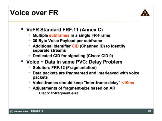
The FRF.11 standard describes how multiple voice communication channels can be transported across a Frame-relay network. The voice channels are packed into separate subframes, of up to 30 byte in length ,with an additional FRF.11 header in front of them. The FRF.11 header carries a Channel ID (CID) which is needed to distinguish between the different voice channels. Several subframes can be transported by one Frame-relay frame depending on the maximum allowed frame size.
