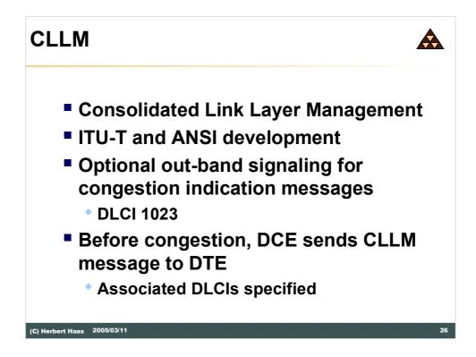
The Consolidated Link Layer Management was developed by the ITU-T and ANSI to provide a more sophisticated tool for congestion indication.
