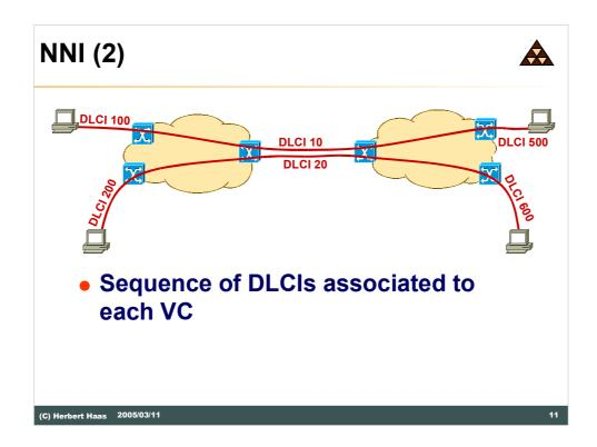
By the use of the Frame-relay NNI interface a sequence of DLCI's is established which represent the virtual connection. This means the connection between two FR-DTE's with each other is determined by a sequence of DLCI's like in our example DLCI 200 - 20 - 600.
