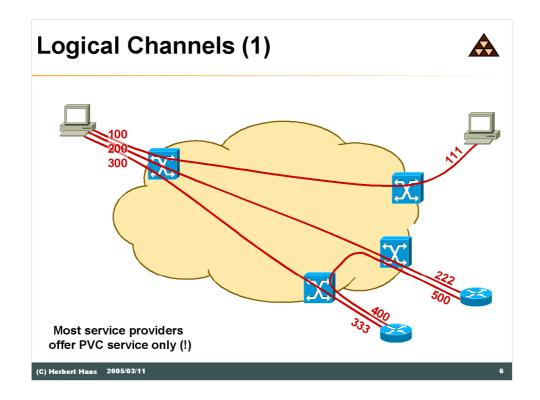
Frame-relay is using virtual circuit identifiers to build up logical channels on one and the same physical Frame-relay connection. The virtual identifiers have local meaning only, that means the must be unique per physical connection only.
