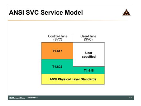
The ANSI T1.602 standard is equivalent to the ITU-T Q922 core + upper standard and supports the reliable transport of signaling messages to set up Frame-relay SVC's.
