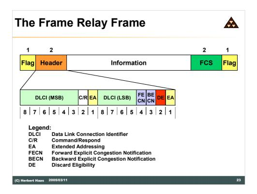
The DLCI field length is typically 10 bits. Optionally, it can be extended using the EA bit (max 16 bits according FRF and GOF). The EA bits are used such that the first and middle DLCI address octets are indicated by EA=0 whereas the last address octet is indicated by EA=1.
