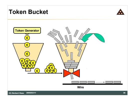
The token bucket method consists of a token bucket and a data bucket. The valve of the data bucket, which controls the amount of data that can be sent out, can only be opened by inserting a token. This means data can only be sent if there are tokens available in the token bucket.
