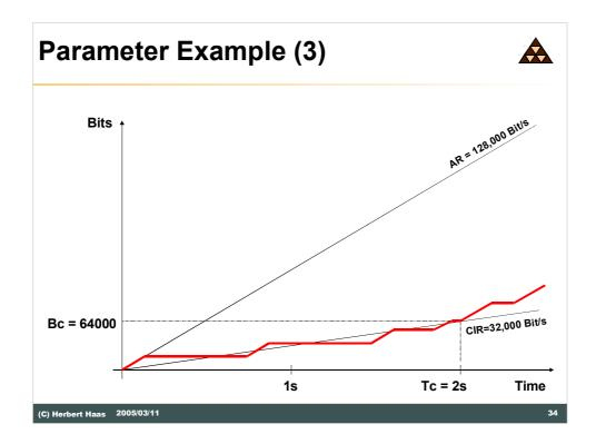
This example shows a more realistic scenario with a lot of small data bursts which in sum do not exceed the CIR. Actually router manufactures use a burst interval much smaller than the Tc. For example a cisco router per default would send out small data burst every 125 milliseconds on a Frame-relay connection. The maximum size of these bursts is calculated from the parameters Tc, Bc, Be and AR which are defined in the traffic contract.
