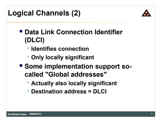
The virtual circuit identifiers are called Data Link Connection Identifiers (DLCI) in Frame-relay technique. Ten bit in the Frame-relay header are reserved for the DLCI, so up to 1024 different DLCI values are possible. Some of them are reserved by the different standards for signaling and congestion indication.
