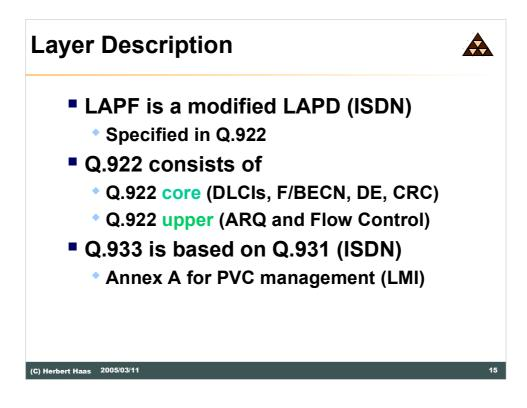
The Link Access Procedure Frame-relay (LAPF) is a modified variant of the Link Access Procedure D-channel (LAPD) used on the D-channel by ISDN to reliable transport Q931 signaling messages.
