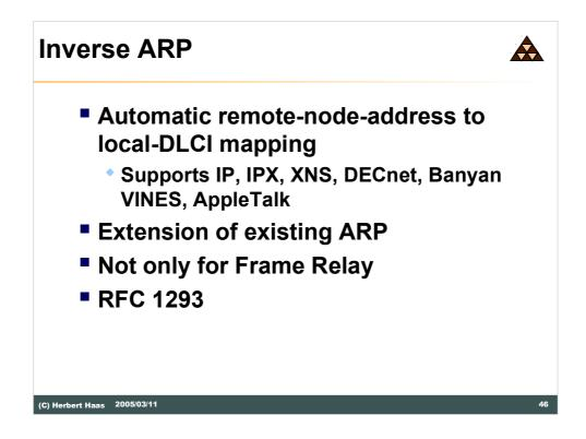
If a layer 3 protocol like IP, IPX, XNS, etc. is transported via a Frame-relay connection layer 2 to layer 3 address mapping needs to be done. The layer 2 address might be a DLCI number in case of PVC service or a E164/X121 address in case of SVC service.
