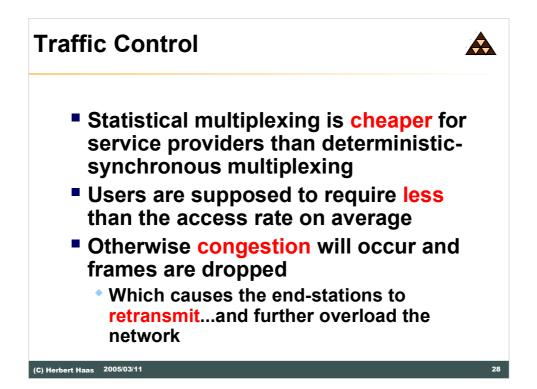
The traffic control in Frame-relay is based on statistical TDM where connections are typically dimensioned on the average traffic needs of all connected users. The service providers try to take advantage of the users traffic behavior, because its very unlikely that all users at the same time use their complete access rate towards the provider.
