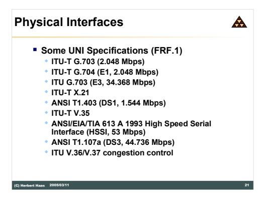
Frame-relay is a typical Data-link technology which can be used on top of many different layer 1 techniques. In this graphic a short overview of the most common used layer 1 techniques in combination with Frame-relay is shown.
