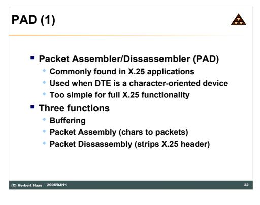
The "Packet Assembler/Dissassembler" (PAD) is an optional device and necessary to connect a dumb asynchronous (character-oriented) device to the X.25 network. The PAD converts the byte-stream into an X.25 packet.
