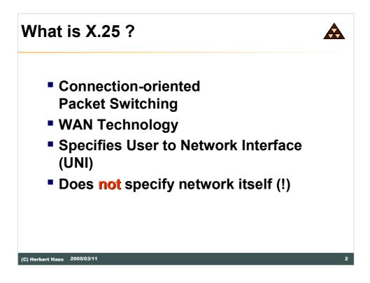
X.25 is wide area network service which is based on the virtual circuit technique. X.25 works only as a user to network interface (X.25 - DTE (e.g. router)  $\leftarrow \rightarrow$  X.25 - DCE (packet switch)). So its connection oriented and based on the store-and-forward principle of packets (packet switching technology).
