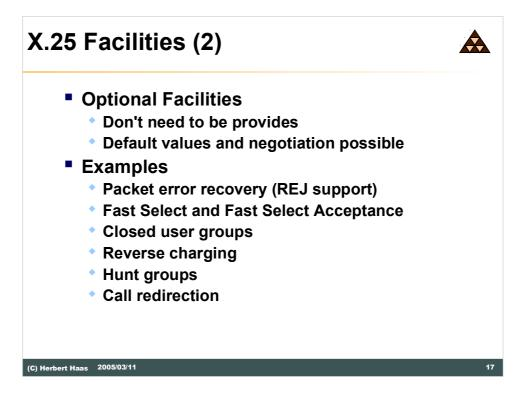
Negotiation of optional facilities can be done in advance between user and service provider, by online-registration or during call setup.
