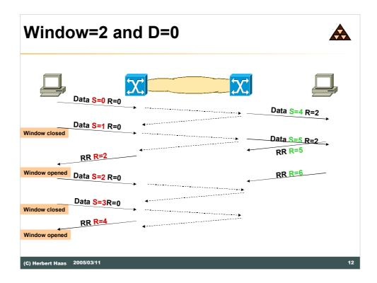
The above example shows an X.25 communication example without using the D bit. Here, data is reliably sent from the left PC (DTE) to the left switch (DCE) and from the left switch to the right (remote) switch. But as soon as a packet arrives on the remote switch, an acknowledgement is generated—actually there is no guarantee that this packet will arrive on the right PC (DTE). But in normal cases, the local link DTE-DCE is reliable enough because of LAPB.
