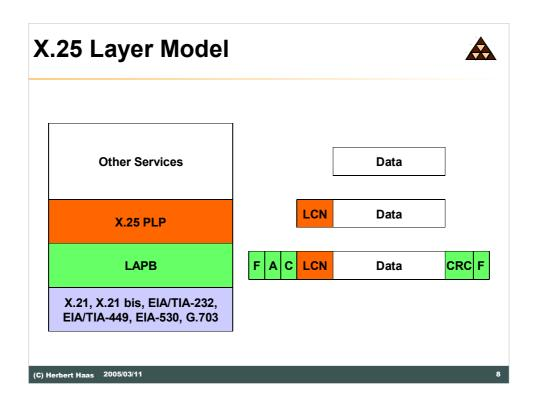
Several physical layer standards have been specified for X.25. One of the most important is X.21bis which defines mechanical and electrical interface issues. Using X.21bis allows synchronous transmission of data up to 19.2 Kbit/s.
