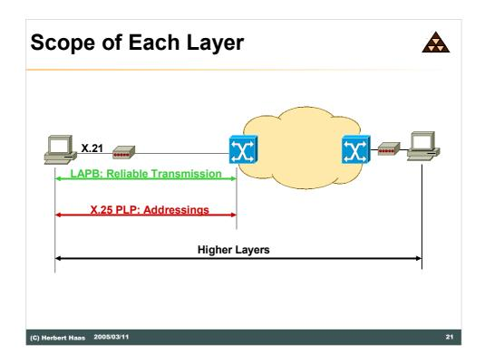
The picture above shows the basic idea and usage of X.25. Higher layer data is carried in X.25 packets that identify the associated virtual calls using a unique address information upon call set-up and LCNs afterwards. LAPB does not differentiate between virtual calls and therefore handles all packets equally. Remember that X.25 is an interface specification only (a UNI) and the internals of the "X.25 network" are not specified.
