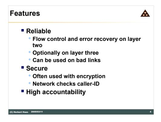
X.25 technology was developed for low quality, low speed lines. Because X.25 use error recovery and flow control on layer 2 to control transmission of frames over physical lines and also use flow control and optionally error recovery on layer 3 to control transmission of packets over a virtual circuit, X.25 is very safe and can be used on very bad links. X.25 is world wide available and mostly used for transaction today (Visa).
