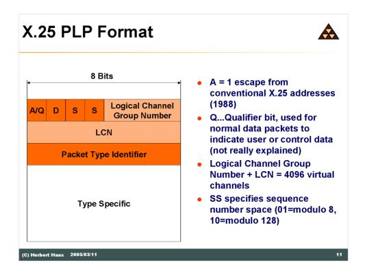
For example the Q-bit can is used for separating X.29 control information for PAD equipment, or QLLC header indication for SNA over X.25.
