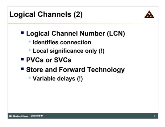
On of the most important things of X.25 is the logical channel number (LCN). Virtual circuits are identified using these LCN numbers, which identifies the connection.
