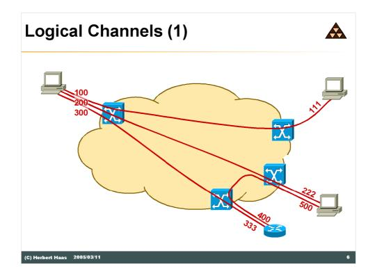
In the picture above you see the virtual circuit principle of X.25. For statistically multiplexing many logical data conversations were build over a single physical transmission link. With X.25 a user build a "virtual pipe" to the destination host.
