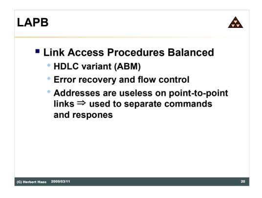
Since LAPB utilizes the ABM mode there is no master/slave relationship. The P/F bit is used for check pointing purposes only, in cases when either end becomes unsure about proper frame sequencing because of a possible missing acknowledgement.
