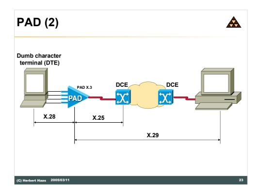
X.28 defines communication issues between a non-packet DTE and a PAD. X.29 defines how a PAD and a remote packet station may exchange control information. The remote station can be a packet-DTE or also a PAD. X.29 identifies these control packets using the Q-bit in the X.25 PLP header. Note that the X.29 protocol allows the configuration of a remote PAD.
