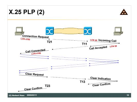
The above picture shows the basic call establishment procedure which is the task of layer 3 (X.25 PLP). Note that this layer is responsible for logical channel numbers so the X.25 PLP cares for (de)multiplexing of different virtual calls over the same physical media.
