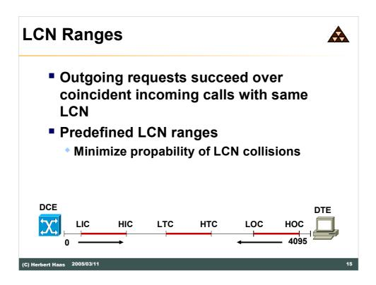
Three ranges can be predefined by the provider to avoid collisions. Two threshold markers are associated to each range. These are:
