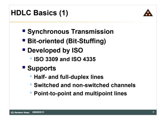
HDLC standardization was done by ISO. HDLC covers a broad range of applications. Therefore HDLC has been used as a basis for a number of other data link layer protocols.
