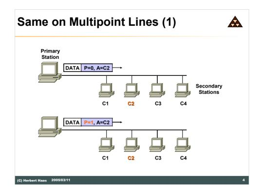
The same principle also works on multipoint lines. In the picture above you see a primary station (server) and 4 secondary stations (hosts) on a multipoint line. The server sends out his date with P=0 to host 2 (C2). When the server is finished with sending data, and when he wants to receive data from C2 he sets the P-bit to 1.
