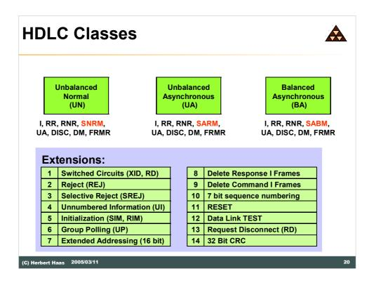
HDLC Classes were created to provide building blocks for implementers. Each HDLC application is one of the three main classes (UN, UA, and BA) and may be provided with extended functionality. For example BA 1.2.3.7.14 means that our application uses combined stations in a full duplex mode using reject and selective reject frames, extended addressing, and 32 bit CRC protection.
