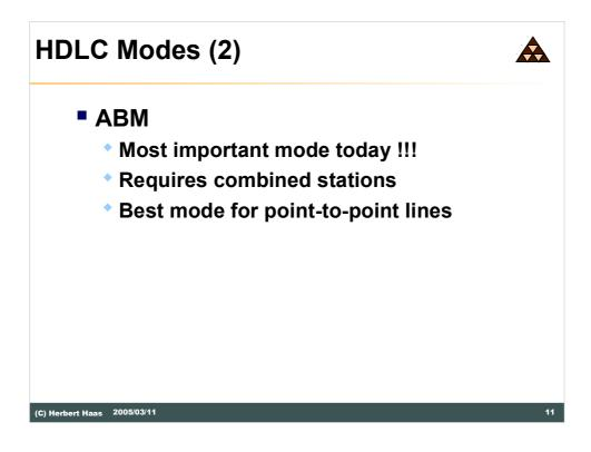
**ABM** is the most important HDLC mode today and is commonly used with full duplex lines – but this is not a requirement. On half-duplex links each station additionally requires some sort of collision-avoidance algorithm. The most important application for ABM is IEEE 802.2 which is used for all important LAN protocols.
