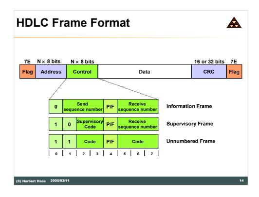
The framing pattern is 0x7E or 01111110 in binary notation. Typically the address field is 8 or 16 bits and also the control field is 8 or 16 bits.
