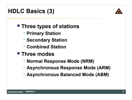
**Primary Station** is responsible for line management, hereby controlling the data flow to/from all stations on the link. There is only one primary station on the link! Secondary frames are called responses.
