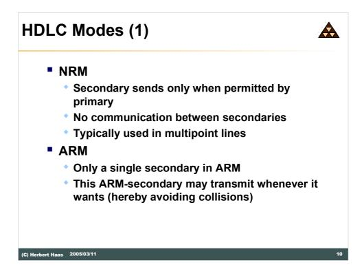
The **NRM** is the oldest mode and is nearly identical with SDLC operation.
