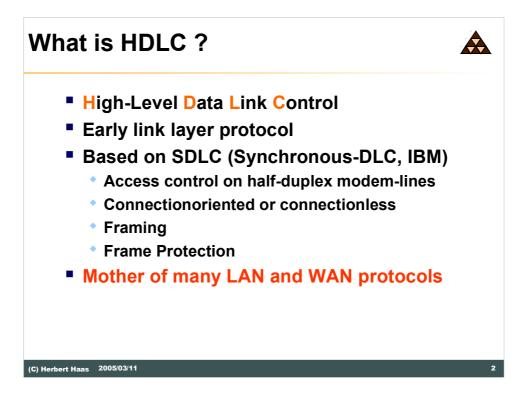
SDLC was created in the mid-1970s to carry SNA (Systems Network Architecture) traffic and supports line speeds up to 64 kbit/s. It was the first bit-oriented synchronous link-layer protocol. SDLC is used for DLSw and Advanced Peer-to-Peer Networking (APPN). ISO adopted and modified SDLC and called it HDLC.
