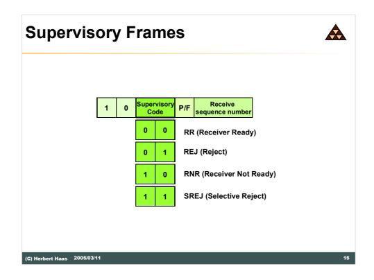
The Supervisory Frames are also called "S-Frames" and are used for error recovery and flow control.
