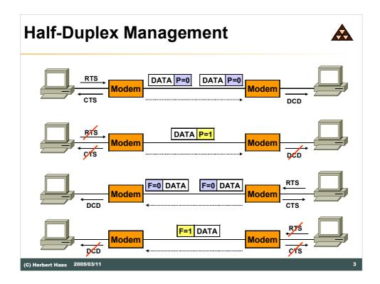
HDLC was created to work in Half-Duplex mode only. The most important thing in the earlier days of HDLC was the P/F bit. This bit was used to hand-over the send-rights.
