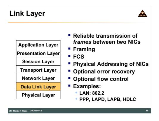
The data link layer builds the frame. In that way, framing or frame synchronization is the most important thing on layer 2. Where is the beginning of the frame ? Where is the end ? With a special Bit-Code the layer 2 protocols, such as HDLC or PPP, guarantee the framing of the data. That's important for the MTU (maximum transfer unit).
