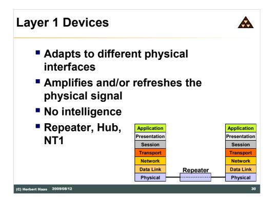
To connect different system with each other we need special devices. If you want to connect two systems only per physical layer you need a so called "hub" or "repeater".
