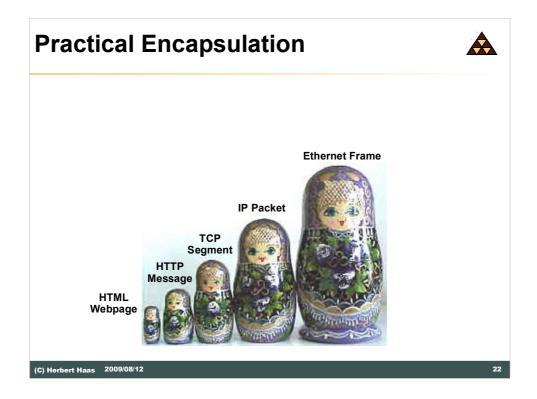
The idea of encapsulation is fundamental in the data communication world. Adjacent layers encapsulate or decapsulate information by adding/removing additional "overheads" or "headers" in order to implement layer-specific functionalities. The whole process can be regarded as Matroschka-puppet principle.
