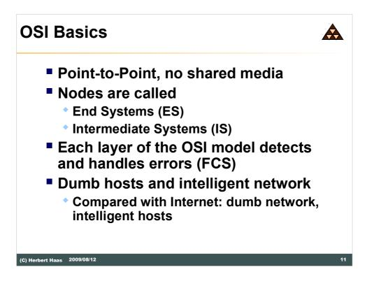
The original OSI modes was created for point-to-point connections only (for example there was no specification for LAN-like shared media originally).
