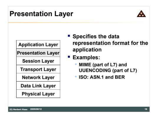
The layer 6 is responsible for common language between end systems. The presentation layer specifies the "meaning" of the data and how each byte should be interpreted.
