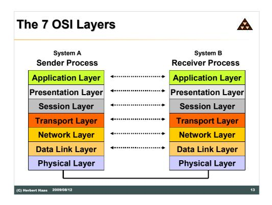
Because the communication between different systems can be a very complex task, OSI splits the communication aspects into smaller tasks. All layering is based on the OSI reference Model, which defines tasks and interactions of seven layers.
