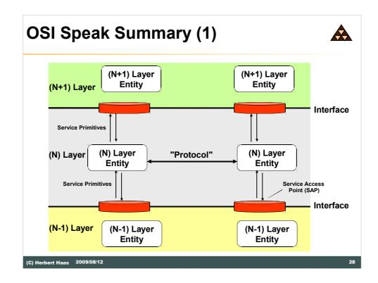
The ISO/OSI model defines four service primitives: request, indication, response and confirm.
