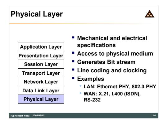
The Physical Layer generates the bit stream. This layer provides access to the physical medium by applying line coding (NRZ, Manchester, etc), synchronization (clocking, PLL), but also includes mechanical specifications. Layer 1 also can activate or deactivate the links between end systems (link management).
