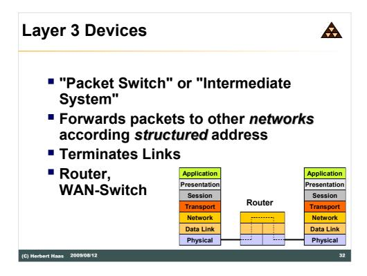
The most important device in the Internet is the so called "router". A router consists of several layer 1 and layer 2 entities and a single layer 3 entity, thus it can forward packets to other networks according structured addresses (remember IP-Addresses). By terminating layer 1 and 2 a router is able to connect total different network technologies with each other. For example: on one side there is Ethernet on the other side ATM.
