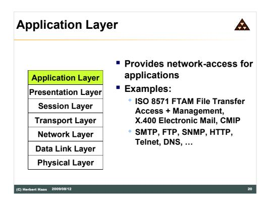
The Application layer supports user with common network applications. For example: file transfer or virtual terminals. Layer 7 also supports basic network procedures in order to implement distributed applications (e.g. transaction systems). Note that the application layer is not identical with the application! The application itself "sits" upon the application layer and uses the service primitives provided by the application layer to access the network.
