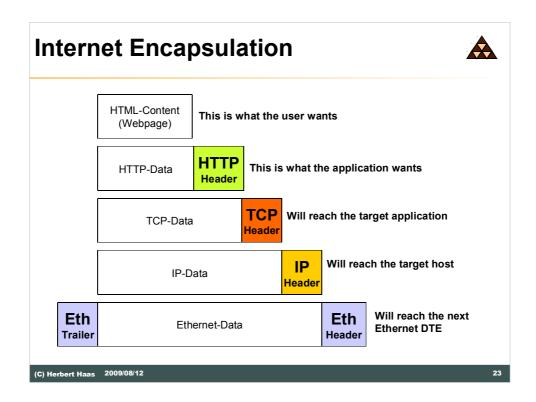
In our example let's suppose a webserver sends a webpage (HTML code) to a client. The webpage is carried via the Hyper Text Transfer Protocol (HTTP) which provides for error and status messages, encoding styles and other things. The HTTP header and body is carried via TCP segments, which are sent via IP packets. On some links in-between, the IP packets might be carried inside Ethernet frames.
