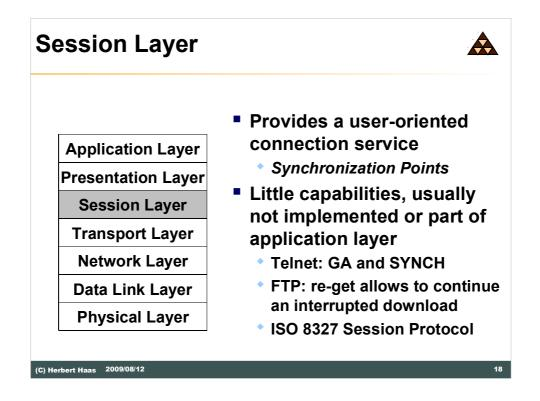
The Session Layer coordinates and controls dialogue between different end systems. This layer is only seldom or sparsely implemented. For example a Telnet server gives the sending permission to the Telnet client via a Go Ahead (GA) sequence. Using the BRK-Key, a SYNCH sequence is triggered and the server must synchronize with the client by flushing the buffered stream. FTP keeps track of the data blocks transmitted and is able to continue an interrupted session from this checkpoint on.
