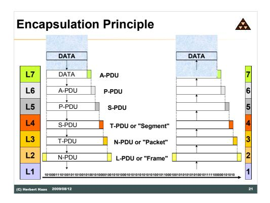
The data moves through all 7 layers. Every layer add his own header. The data with layer 4,5,6 and 7 header is called "segment". A segment plus layer 3 header is called "packet". The so called "frame" (data plus six headers) will be transport over layer 1 to the destination system. Then the frame will moves through all 7 layers again, and in each station a header will be removed.
