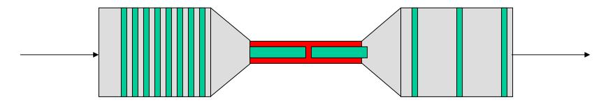
Pipe modell of a network path: Big fat pipes (high data rates) outside, a bottleneck link in the middle. The green packets are sent at the maximum achievable rate so that the interpacket delay is almost zero at the bottleneck link; however there is a significant interpacket gap in the fat pipes.
