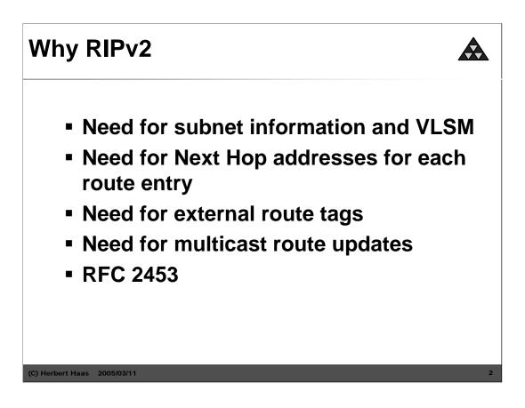
Because Subnetting and VLSM get more important RIPv2 was created. RIPv2 was introduced in RFC 1388, "RIP Version 2 Carrying Additional Information", January 1993. This RFC was obsolete in 1994 by RFC 1723 and finally RFC 2453 is the final document about RIPv2.
