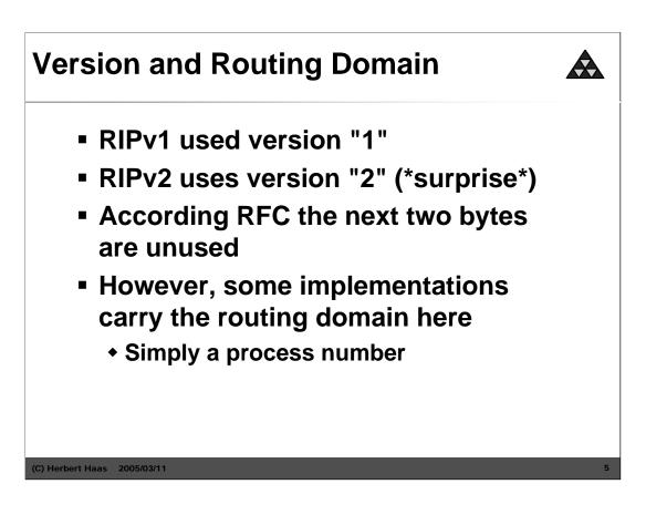
The routing domain indicates the routing-process for which the routing-update is destined. Now routers can support several domains within the same subnet.
