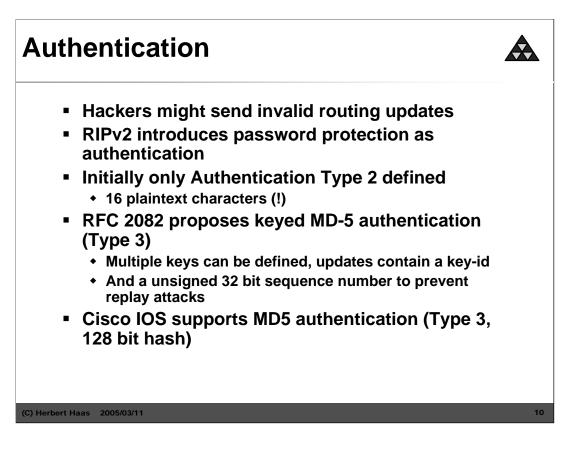
IF a router receives routing updates without valid authentication are ignored by the receiving router, because only trusted router are accepted.
