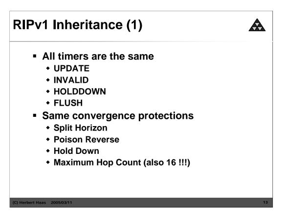
RIPv1 uses many timers to regulate its performance. This timers are the same in RIPv2. The routing update timer is set to 30 seconds, with a small random amount of time added whenever the timer is reset. A route is declared invalid without being refreshed by routing updates during 90 seconds. The "holddown" status retains 180 seconds. In this time a router ignore update messages about a special network. After 240 Seconds (Flush timer) a non-refreshed routing table entry will be removed.
