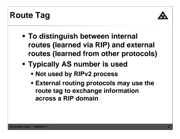
Route Tag contains the autonomous system number for EGP and BGP. When the router receive a routing-update with a routing tag unequal zero, the associated path must be
