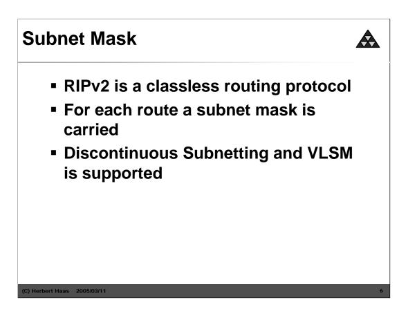
Remember RIP is an classful routing protocol, because RIPv1 does not bind subnet-masks to the routes. So RIPv1 assumes classful addressing.
