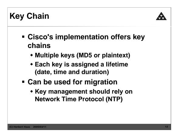
Several independent routing domains running RIPv2 with different process numbers ("routing domain"). With using key chains this domains can be work together (synchronize) at a special time or date.
