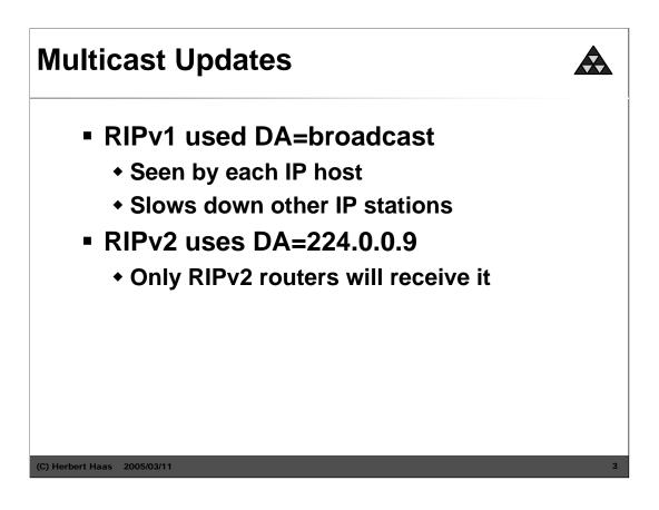
RIPv2 uses the IP-Address 224.0.0.9 to transfer his routing updates. With this advantage only RIPv2 routers see this messages, and will not slow down the different station (RIPv1 and broadcast addresses).
