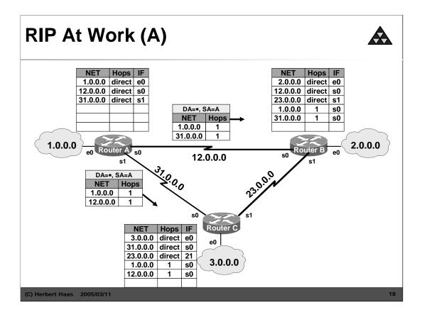
Split Horizon at work: Router A didn't tell router B about the network 12 and router A didn't tell router C about the network 31, because the router knows that router B must have a direct connection to network 12 and that router C must have a direct connection to network 31.
