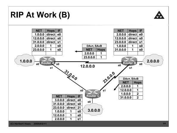
And so router B tells router A only about network 2 and 23 and router C only about network 2 and 12.
