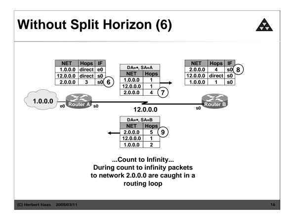
Either router A or router B has information about the Network 2, both router will increase the hop count by 1 every routing update. Count to infinity accurse. Now Update packets are caught in a routing loop.
