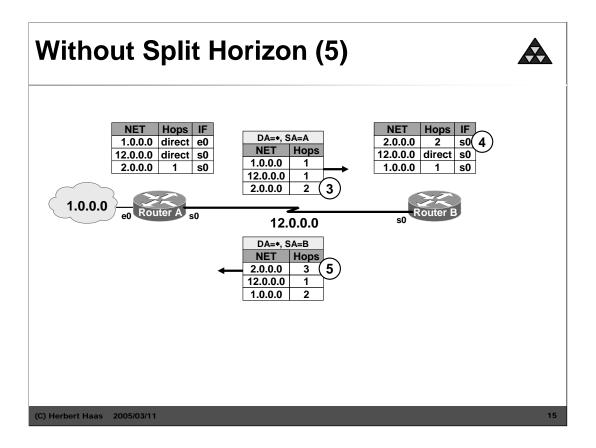
Now router B receives a routing update from router A including reach ability information about network 2. Because router B has no information about network 2 he adds this information in his routing table and continuous sending his normal routing updates to router A, hereby increasing the hop count by 1.
