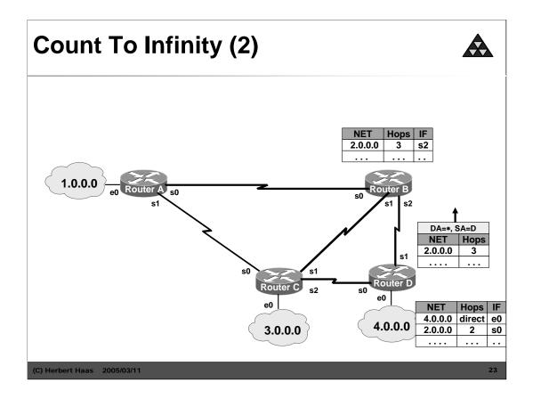
And a new connection established between router B and router D. Now, a normal routing update is send from router D to router B (with information about net 2, of course).
