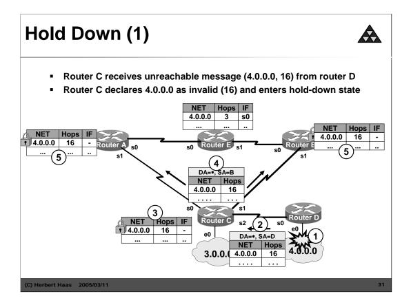
In this example we see the functionary of Hold Down. After Net 4 crashes, router D send this information to Router C. Router C added this information and activate "hold down". After this he sends this information to his neighbor routers, which do the same after they receive the information about net 4.
