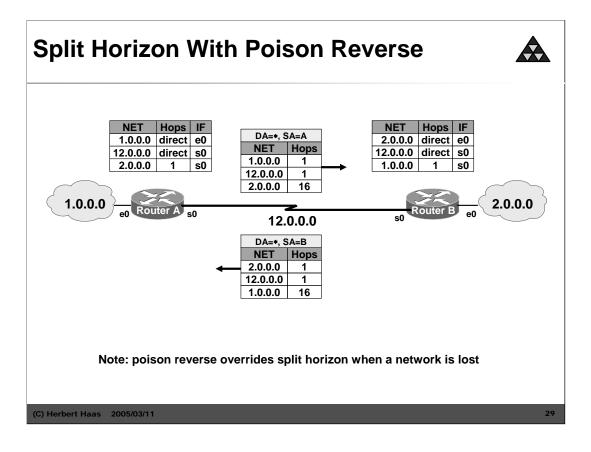
Split horizon with poisoned reverse includes also reverse routes in updates, but sets their metrics to infinity. This is safer than simple split horizon: If two gateways have routes pointing at each other, advertising reverse routes with a metric of 16 will break the loop immediately.
