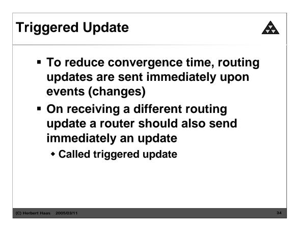
To speed up the convergence time, "**triggered update**" has been introduced. After a router notice a network failure, he immediately sends a routing update to indicate this failure. So the router didn't wait for the expiration of the 30 seconds. Triggered update can used with all events (e.g. a new link established).
