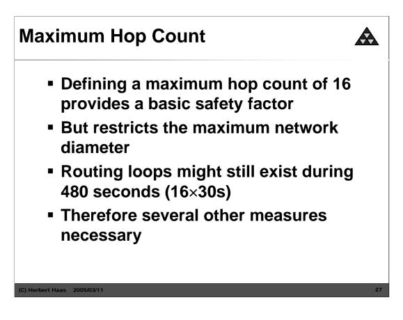
The maximum hop count is a basic safety factor, but it is also the main drawback of RIP. It restrict the maximum network diameter, and the rooting loops exist for 480 seconds. During Count to Infinity there is a bad routing and the network must deal with unnecessary traffic. So we need other measures like Poison Reverse.
