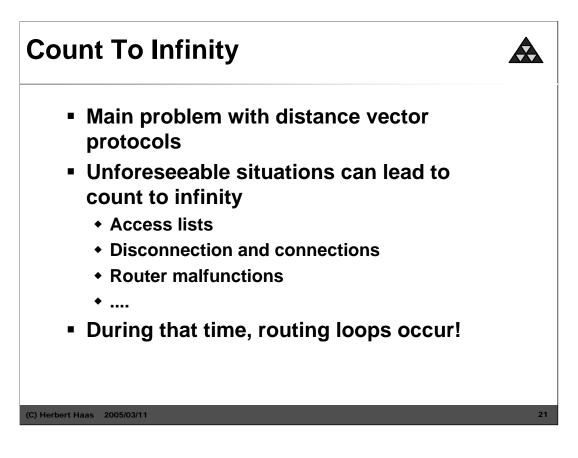
Because of the simple principle of RIP (Distance Vector protocol), we cannot prevent Count to Infinity. Access Lists, Disconnection and connections, Router malfunction, etc can always lead to it, there is no 100% solution.
