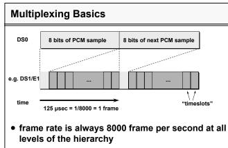
• byte interleaved multiplexing
