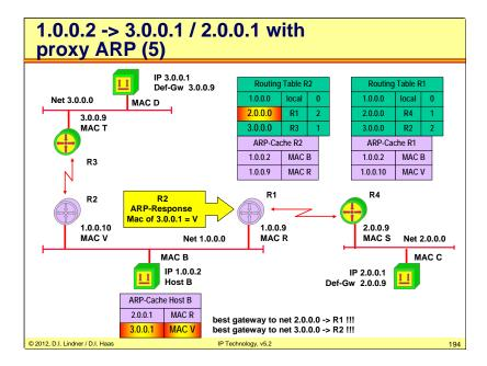
Response of R2 sent to Host B only (ARP reply uses directed addressing)!
