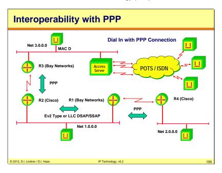
After the interoperability issue was solved PPP focuses on providing dial-in connectivity for IP systems. PPP connections between IP hosts (PCs) and access-servers allow working from remote in the same way as if the IP host would be directly connected to a LAN.
