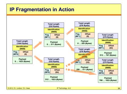
The example above shows how an IP packet (left) is fragmented into two smaller fragments (middle) by a router and further fragmented into a total number of four fragments by a another router (right).
