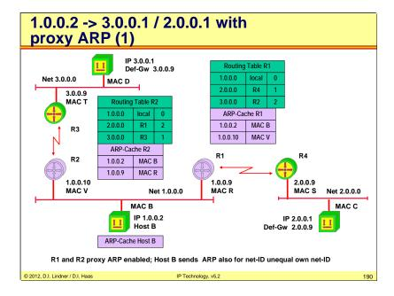
Router R1 and R2 are configured to support proxy ARP (acting as a proxy ARP gateway). Host B is configured to use proxy ARP extension by pointing to its own IP address as default gateway.
