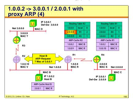
Request is sent to all systems on the given LAN (ARP request uses L2 broadcast addressing)!
