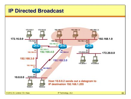
In this example a datagram to the Network 192.168.1.0 is sent but the host-ID is set to "allones". As routers do not care about the host IDs, this datagram is forwarded according its destination network number, and only the last router is responsible for direct delivery.
