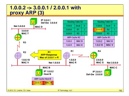
Response of R1 sent to Host B only (ARP reply uses L2 directed addressing)!
