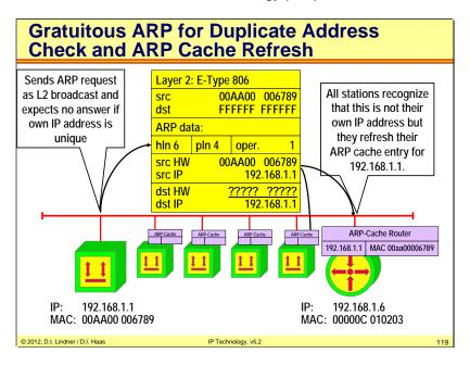
Gratuitous ARP is an ARP request where an IP station asks for address resolution of its own IP address.
