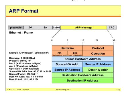
ARP messages are carried within Ethernet II frames or SNAP encapsulation using type field 0x806. ARP has been designed to support different layer 3 protocols (IP is just one of them).
