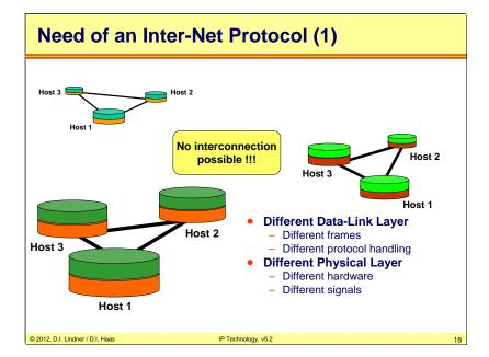
Why do we need an Inter-Net Protocol? Different networks have different Data-Link Layer. Every Network runs a different protocol. Some networks use proprietary link layer protocols or X.25, other networks have Ethernet or HDLC. You see, every network has its own hardware, signals and frames. As long as they do not want to communicate with each other, there is no problem...
