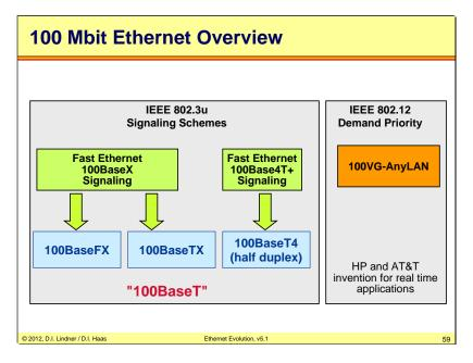
The diagram above gives an overview of 100 Mbit/s Ethernet technologies, which are differentiated into IEEE 802.3u and IEEE 802.12 standards. The IEEE 802.3u defines the widely used Fast Ethernet variants, most importantly those utilizing the 100BaseX signaling scheme. The 100BaseX signaling consists of several details, but basically it utilizes 4B5B block coding over only two pairs of regular Cat 5 twisted pair cables or two strand 50/125 or 62.5/125-µm multimode fiber-optic cables.
