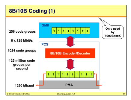
8B10B block coding is very similar to 4B5B block coding but allows fully balanced 10-bit codewords. Actually, there are not enough balanced 10-bit codewords available. Note that there are 256 8-bit codewords which need to be mapped on 1024 10-bit codewords. But instead of using a fully balanced 10-bit codeword for each 8-bit codeword, some 8-bit codewords are represented by two 10-bit codewords, which are sent in an alternating manner. That is, both associated 10-bit words are bit-complementary.
