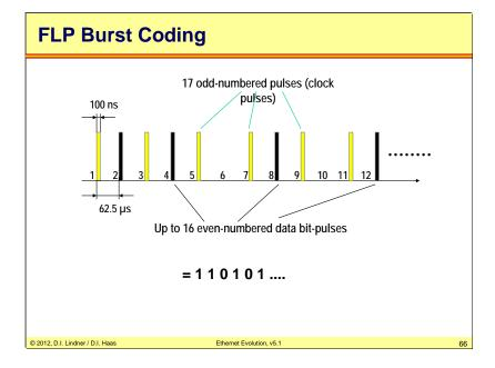
A series of FLPs constitute an autonegotiation frame. The whole frame consists of 33 timeslots, where each odd numbered timeslot consists of a real NLP and each even timeslot is either a NLP or empty, representing 1 or 0. Thus, each FLP sequence consists of a 16 bit word.
