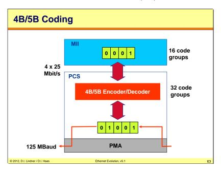
The diagram above shows the basic principle of the 4B5B block coding principle, which is used by 802.3u and also by FDDI. The basic idea is to transform any arbitrary 4 bit word into a (relatively) balanced 5 bit word. This is done by a fast table lookup.
