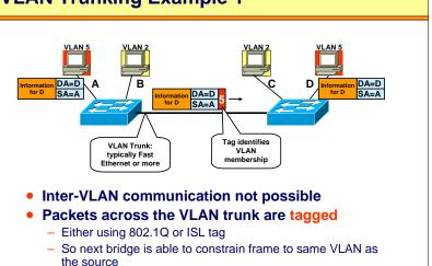
By using VLAN tagging the "next" bridge knows whether the source address is also member of the same VLAN.
