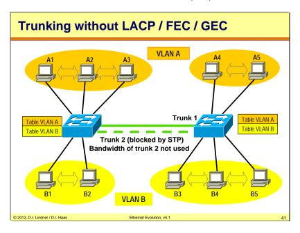
On trunks between multiport switches full duplex operation is used of course. In case of parallel trunks the normal operation of STP will block one trunk link and hence bandwidth of this link can not be used.
