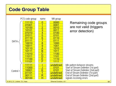
Recognize: Start Delimiter (SD) and End Delimiter (ED) for frame synchronization of an Ethernet frame are coded in control code-points -> that are code-violations in this context. Real data is coded DATA code-points.
