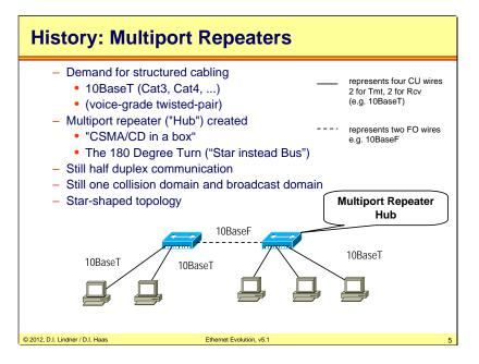
Later, Ethernet devices supporting structured cabling were created in order to reuse the voice-grade twisted-pair cables already installed in buildings. 10BaseT had been specified to support Cat3 cables (voice grade) or better, for example Cat4 (and today Cat5, Cat6, and Cat7).
