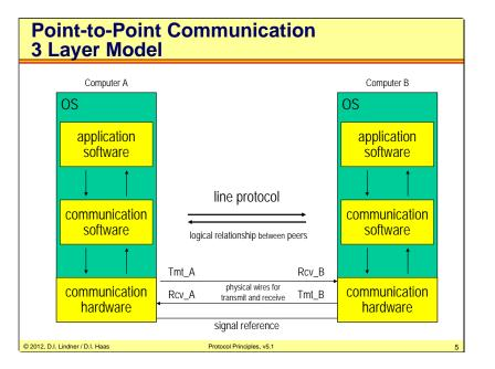
The line protocol is implemented on transit by using the control field / protocol header of a frame. The horizontal arrows describe this logical cooperation between systems. The actual physical transport of bits (frames) is performed by the communication hardware (encoding, bit synchronization, frame synchronization and so on).
