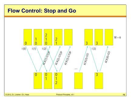
Typically used flow control messages are <u>STOP</u>, e.g. HDLC's Receiver Not Ready (RNR) <u>GO</u>, e.g. HDLC's Receiver Ready (RR)
