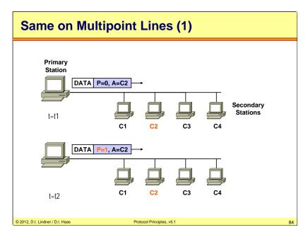
The same principle also works on multipoint lines. In the picture above you see a primary station (server) and 4 secondary stations (hosts) on a multipoint line. The server sends out his date with P=0 to host 2 (C2). When the server is finished with sending data, and when he wants to receive data from C2 he sets the P-bit to 1.
