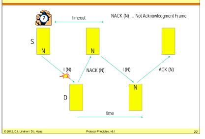
With NACK we need not to wait for the timeout to expire, hence the receiver can trigger the retransmission earlier. The problem for the receiver: How to get noticed about a corrupted frame (usually physical hardware will silently discard a received frame with an CRC-FCS error indicated).
