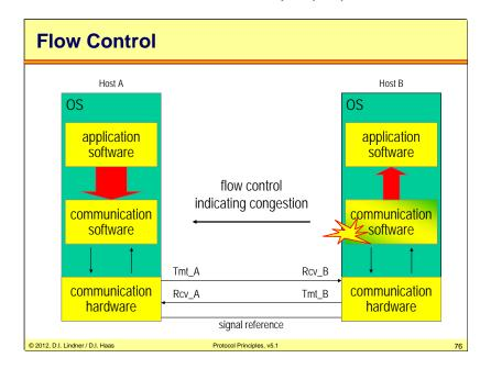
If data frames arrive faster than application is able to process,
