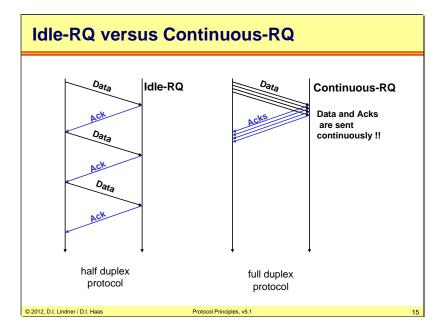
Idle-RQ: After sending a data frame the transmitter must wait for the acknowledgment before next data frame is allowed to send (half duplex protocol).
