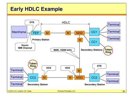
The slide above shows a typical HDLC application. Many terminals which are connected to Cluster Concentrator.
