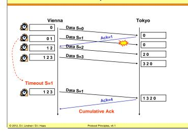
In the positive ARQ technique an ACK is only sent when the order of the arriving data frames is correct.
