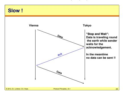
As already mentioned before the idle-RQ technique is not suited for today's data transport systems. The stop and wait procedure would introduce a lot of delay, especially on long distance connections, and would no be able to efficiently use the network infrastructure.
