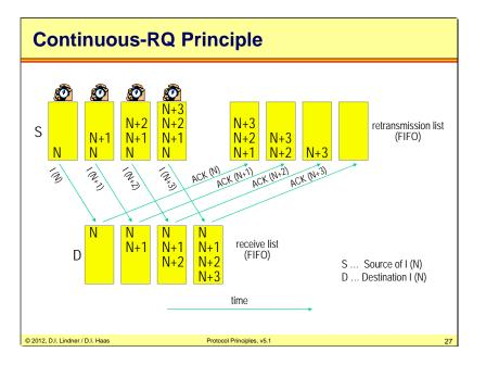
Continuous-RQ protocols were developed for more efficient usage of full duplex lines. Device does not wait for acknowledgements for frames already sent. Full duplex protocol.
