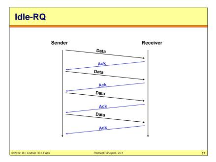
The idle-RQ technique is a stop and go protocol, this means when the sender has sent out one data frame he must wait for the according acknowledgement before he is allowed to sent the next frame.
