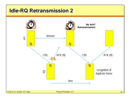
Retransmission caused by loss of a acknowledgement frame (ACK). Receiver needs receive buffer/ receive list to store last correct frame in order to recognize data frame duplicates.
