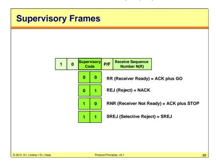
The Supervisory Frames are also called "S-Frames" and are used for error recovery and flow control.
