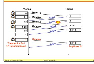
The Selective Acknowledgement technique causes retransmissions even in the case when only the acknowledgement frame is lost. Because if the Ack frame is missing the sender is not allowed to remove the according data frame from the send buffer.
