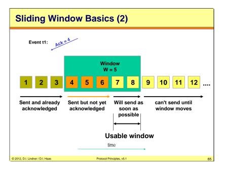
As soon as the first ACK = 4 (t1) arrives the sliding window moves to the left. This is possible because the data frames 1,2 and 3 are now removed out of the send buffer. Now the data frames 4, 5 and 6 are sent and kept in the send buffer until their acknowledgements arrive.
