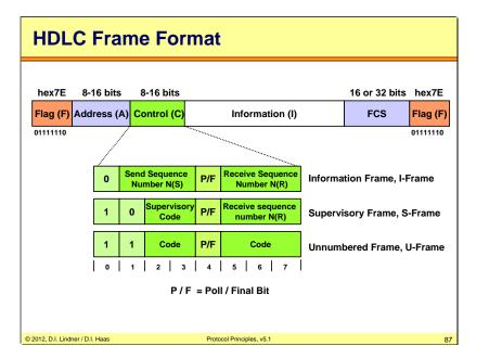
The framing pattern is 0x7E or 01111110 in binary notation. Typically the address field is 8 or 16 bits and also the control field is 8 or 16 bits.
