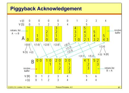
Until now ACKs control frames for received data frame were only seen in one direction (data flow streams in the opposite direction). If there is data flow in both directions dedicated ACK frames produce unnecessary overhead. Therefore acknowledgments contained in data frames in opposite direction can avoid that overhead -> Piggyback Acknowledgement.
