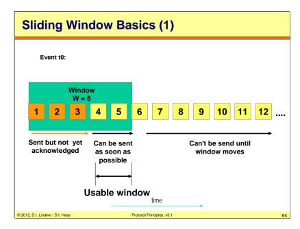
In this example a fixed window size of five is used. This means that up to five data frames without explicit acknowledgments may be sent. At the start time to we sent out three frames.
