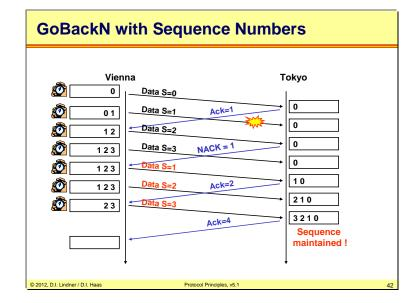
In GoBackN ARQ technique data frames are only acknowledged when the series of received sequence numbers is continuous.
