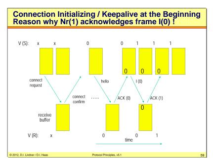
Connection establishment initializes V(S) and V(R) to zero.
