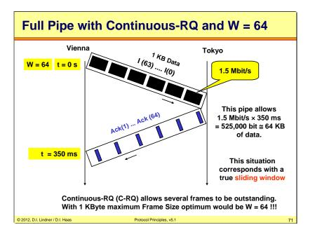
By the use of continuous-RQ technique and an proper adjusted send window size it would now be possible to use the complete capacity of our Vienna – Tokyo connection.
