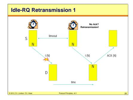
Retransmission caused by loss of a data (information) frame (I).
