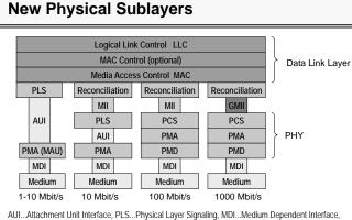
AUI...Attachment Unit Interface, PLS...Physical Layer Signaling, MDI...Medium Dependent Interface, PCS...Physical Coding Sublayer, MI...Media Independent Interface, GMII...Gigabit Media Independent Interface, PMA...Physical Medium Attachment, MAU...Medium Attachment Unit, PMD...Physical Medium Dependent 2006, DL Market Lindner Ethermet Evolution, v4.7 4 L07 - Ethernet Evolution and Wireless LAN Primer
