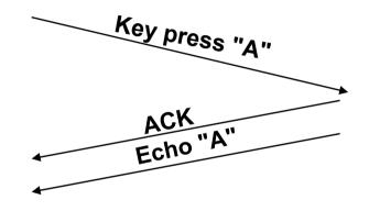
Example: Telnet with Delayed ACK
