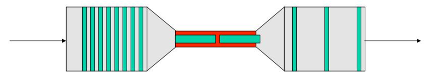
Pipe model of a network path: Big fat pipes (high data rates) outside, a bottleneck link in the middle. The green packets are sent at the maximum achievable rate so that the interpacket delay is almost zero at the bottleneck link; however there is a significant interpacket gap in the fat pipes.
