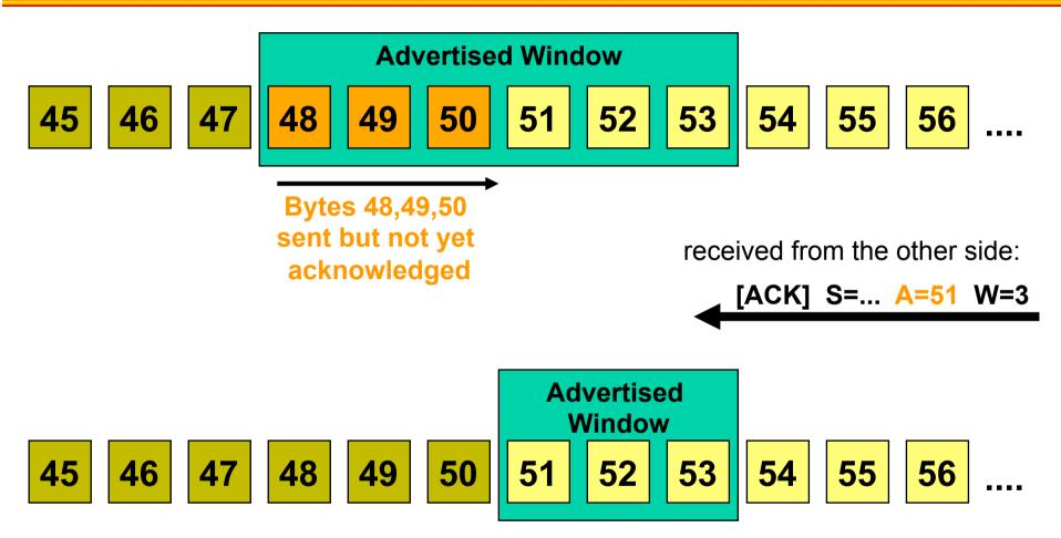
Now the sender may send bytes 51, 52, 53. The receiver didn't open the window (W=3, right edge remains constant) because of congestion. However, the remaining three bytes inside the window are already granted, so the receiver cannot move the right edge leftwards.
