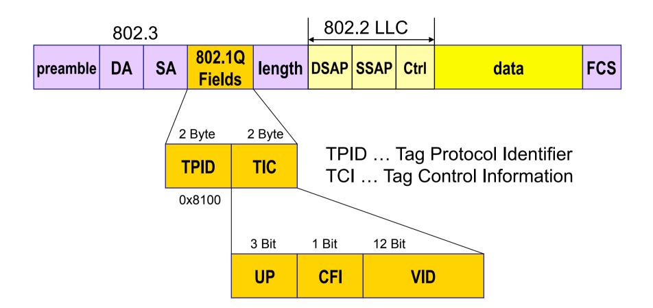
note: With tagging Ethernets maximal frame length = 1522, minimal frame length = 68 UP ... User Priority for L2 QoS = COS CFI ... Canonical Format Identifier VID ... VLAN Identifier
