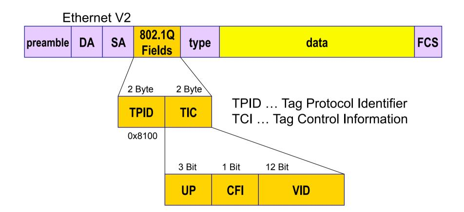
note: With tagging Ethernets maximal frame length = 1522, minimal frame length = 68 UP ... User Priority for L2 QoS = COS CFI ... Canonical Format Identifier VID ... VLAN Identifier
