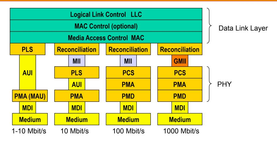
AUI...Attachment Unit Interface, PLS...Physical Layer Signaling, MDI...Medium Dependent Interface, PCS...Physical Coding Sublayer, MII...Media Independent Interface, GMII...Gigabit Media Independent Interface, PMA...Physical Medium Attachment, MAU...Medium Attachment Unit, PMD...Physical Medium Dependent Dependent
