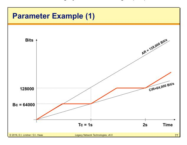
In this example the measurement time interval Tc is set to 1second, the Bc to 64000 bits and the physical access rate is 128 Kbit/s. The red line indicates the actual traffic pattern used on this connection. In this scenario the traffic characteristic remains within the CIR of 64 Kbit/s.
