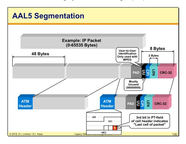
The Common Part Indicator (CPI) is not really used until today, so all 8 bits are set to zero. Most interestingly, the length field is 16 bits that is 64 KByte packets are supported. So, ATM is one of the few technologies that support maximum IP packet sizes (IP also supports up to 65535 Bytes per packet).
