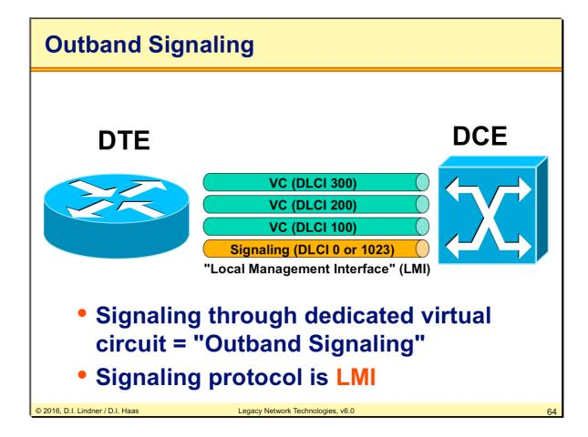
The Local Management Interface (LMI) was developed to inform the Frame-relay users about the condition of the Frame-relay network itself.
