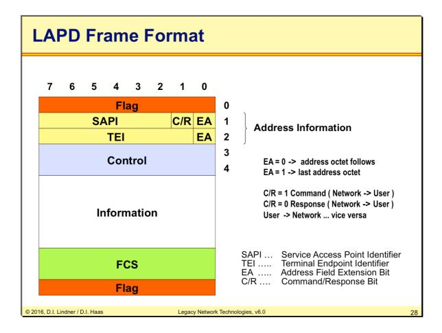
The picture above shows the Q.921 or LAPD frame format. The Service Access Point Identifier (SAPI) and the Terminal Endpoint Identifier (TEI) are described next.
