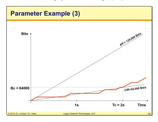
This example shows a more realistic scenario with a lot of small data bursts which in sum do not exceed the CIR. Actually router manufactures use a burst interval much smaller than the Tc. For example a Cisco router per default would send out small data burst every 125 milliseconds on a Frame-relay connection. The maximum size of these bursts is calculated from the parameters Tc, Bc, Be and AR which are defined in the traffic contract.
