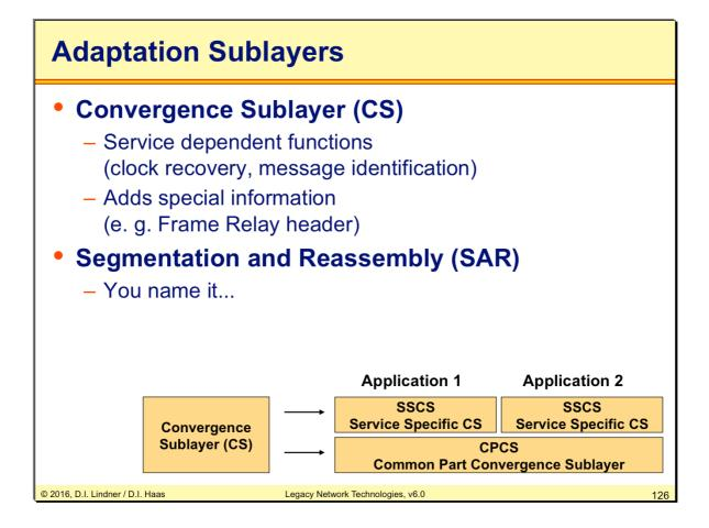
The Convergence Sublayer (CS) is divided in two further sublayers, the Common Part Convergence Sublayer (CPCS) and the Service Specific Convergence Sublayer (SSCS). The CPCS is common to all instances of a specific AAL. Therefore only one CPCS has been defined per AAL while many SSCS can be defined for the same AAL.
