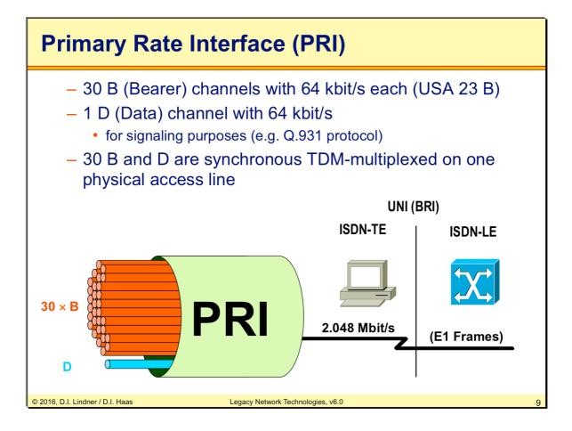
The PRI also contains B and D channels, but now there are 30 B channels and also the D channel has the same bandwidth of 64 kbit/s. These 31 channels plus an additional synchronization channel result in a total data rate of 2,048 Mbit/s, which is transported over a E1 frame (basic component of PDH hierarchy).
