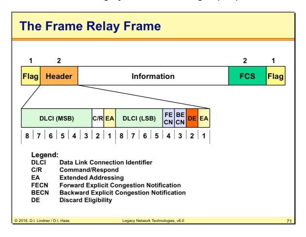
The DLCI field length is typically 10 bits. Optionally, it can be extended using the EA bit (max 16 bits according FRF and GOF). The EA bits are used such that the first and middle DLCI address octets are indicated by EA=0 whereas the last address octet is indicated by EA=1.
