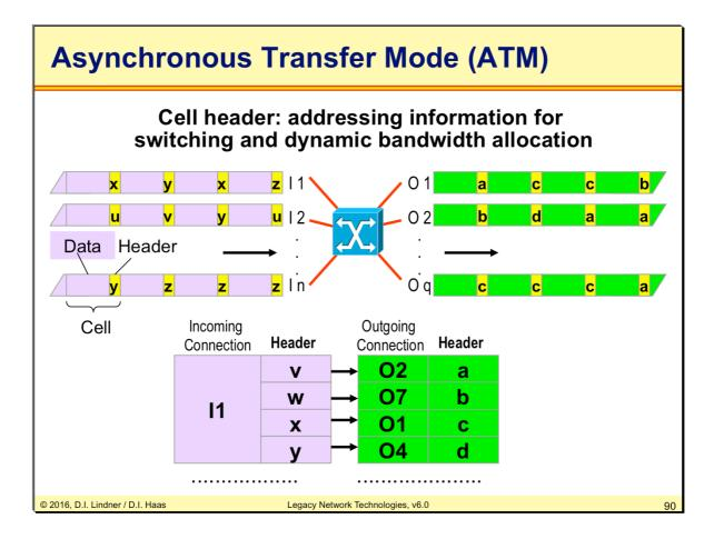
This pictures just shows again the principle of packet switching in the connection-oriented mode by using local connection identifier information (contained in the cell protocol header) to decide based on the switching table where to move on a packet (cell) and swapping the local connection identifier for usage on the next outgoing line.
