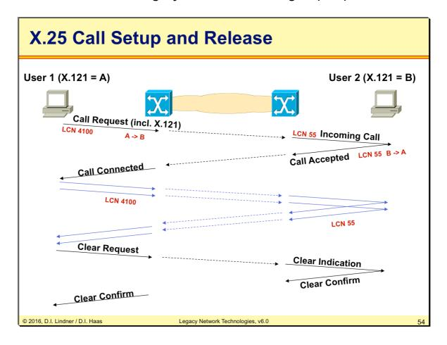
The above picture shows the basic call establishment procedure which is the task of layer 3 (X. 25 PLP). Note that this layer is responsible for logical channel numbers so the X.25 PLP cares for (de)multiplexing of different virtual calls over the same physical media.
