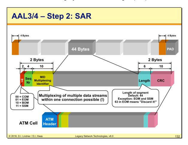
The sequence number enumerates each 44 byte segment of the CS frame (modulo 16). The Multiplexing Identifier (MID) allows to multiplex up to 210 different connection-oriented AAL 3/4 connections. For connectionless packets, the MID field can be used as unique identifier associated with each user, in order to multiplex many users over one ATM pipe.
