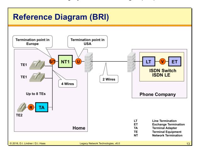
A TE2 is for example a plain old telephone (POT) or an analog modem. The R interface is typically a EIA/TIA-232-C, V.24, or V.35.
