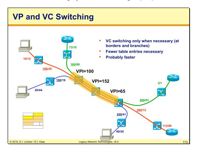
If one customer asks for another 100 virtual circuits, the provider does not need to add 100 additional entries in every switching table—as he must do with Frame Relay for example—because one VPI represents a number of VCIs and inside the network VPI switching is performed.
