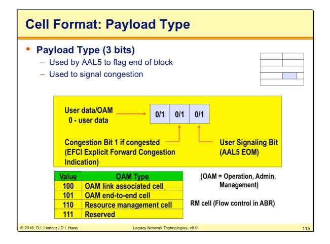
The Payload Type (PT) is used to identify the cell payload (OAM, Resource Management, ...) EFCI has the same meaning und purpose as the FECN of frame relay -> congestion indication to the receiving side.
