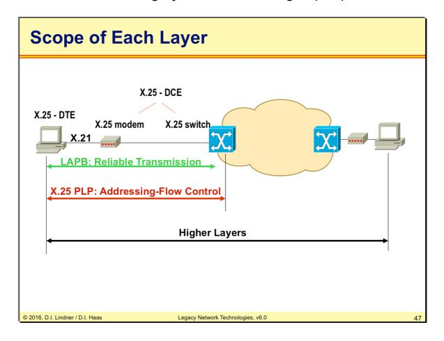
The picture above shows the basic idea and usage of X.25. Higher layer data is carried in X.25 packets that identify the associated virtual circuits using a unique address information (X.121) upon call set-up and LCNs afterwards. LAPB does not differentiate between virtual circuits and therefore handles all packets equally.
