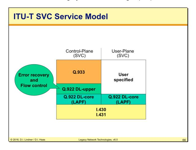
But Frame Relay can also support SVC services. In this case we don't use Annex A but rather plain "Q.933". Furthermore SVC mode requires a reliable Q.922 connection to the DCE, which is handled by the so-called "Q.922 DL-upper". The Frame Relay layer itself is the Q.022 DL-core layer, which must be always existent.
