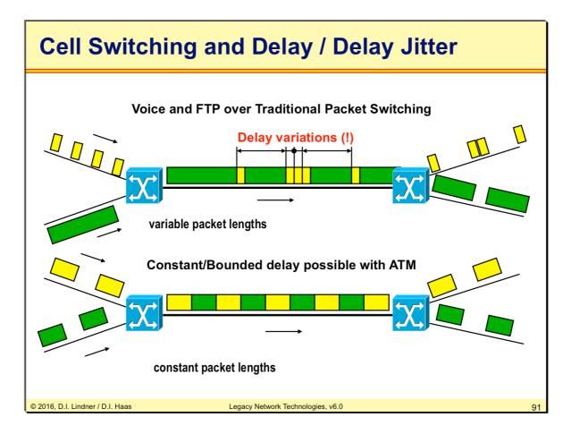
Jitter is change in inter-arrival times between cells/packets.
