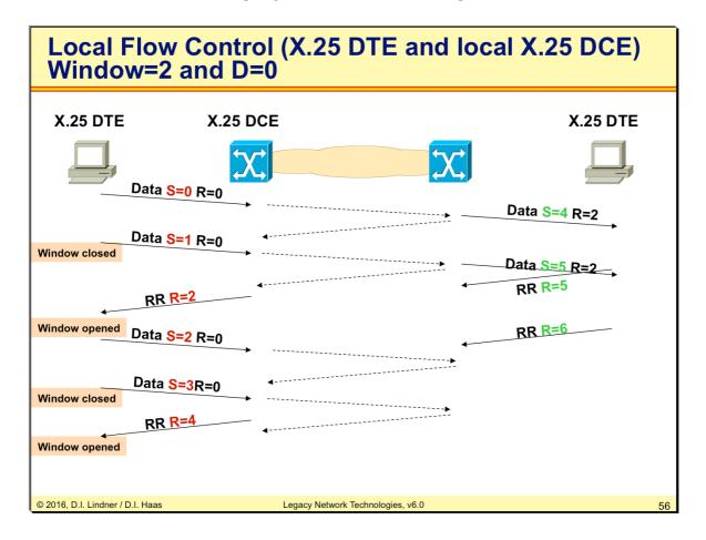
Flow control is based on windowing and PLP RNR (RR) messages. Upon delay of acknowledgment, the receiver closes the send window of the sender (windowing). The default window size is 2. Optional end-to-end error recovery (GoBack N) can be achieved using the D-bit in the X.25 PLP header.
