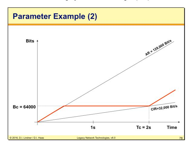
In this scenario a measurement interval Tc of 2 seconds is chosen. The committed burst size Bc is 64000 bits, so the CIR according to the formula CIR = Bc / Tc will be 32 Kbit/s. The actual traffic pattern indicated by the red line remains again within the borders of the CIR.
