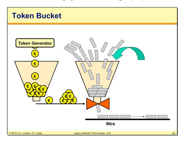
The token bucket method consists of a token bucket and a data bucket. The valve of the data bucket, which controls the amount of data that can be sent out, can only be opened by inserting a token. This means data can only be sent if there are tokens available in the token bucket.
