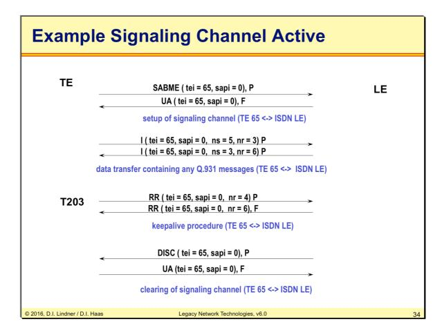
This picture shows an example for a setup, data transfer and tear down of a LAPD connection used by a TE to reliable transport signaling messages carried by LAPD I frames to the LE.
