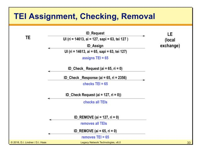
This picture shows an example for TEI management carried by UI frames of LAPD performed between TE and LE.
