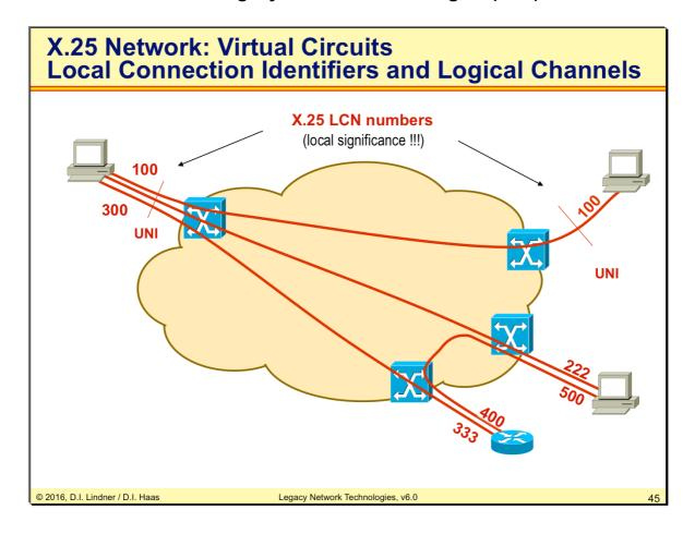
In the picture above you see the virtual circuit principle of X.25. With statistically multiplexing many logical data conversations were build over a single physical transmission link. With X.25 a user build a "virtual pipe" to the destination host.
