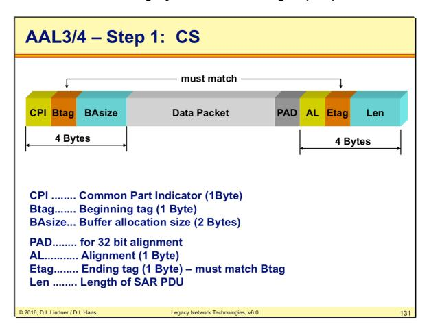
CPI indicates the interpretation of the remaining fields. Currently only value zero is defined which indicates that the values in BAsize and Length should be interpreted as amount of bytes.
