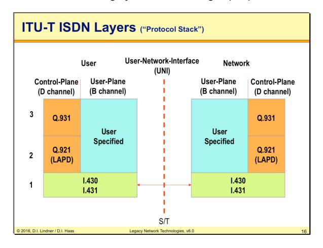
The diagram above shows the ISDN layer model. There is one common physical layer, which is either I.430 (the BRI) or I.431 (the PRI). Note the vertical separation above the common physical layer - a clear sign of outband signaling!
