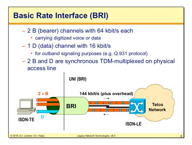
The picture above describes the BRI which might be installed in every household. The BRI specifies three channels: 2 Bearer (B) channels providing 64 kbit/s each and one signaling or Data (D) channel, providing only 16 kbit/s.
