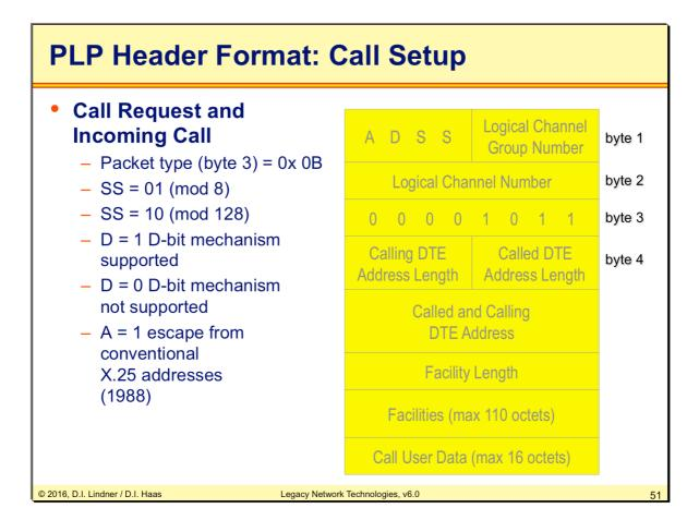
Called and Calling DTE Address are the unique and structured X.121 addresses (L3 addresses) which allows a worldwide public X.25 service like the good old telephony service.
