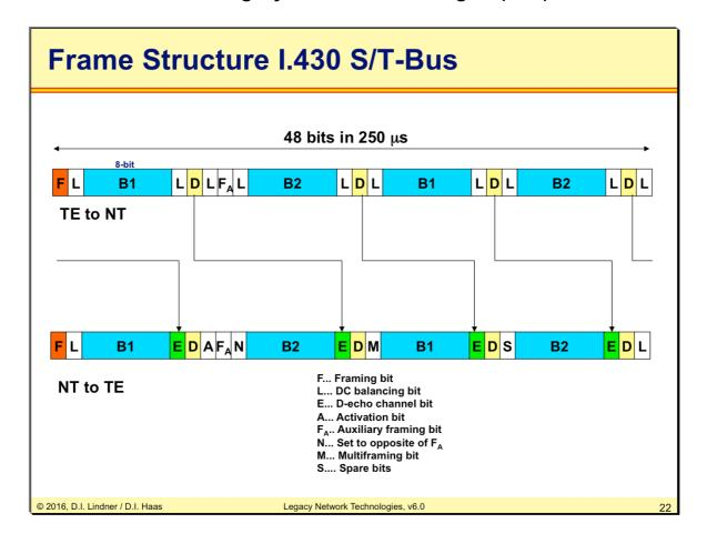
Frame of 48 bit is transmitted in a period of 250 usec.
