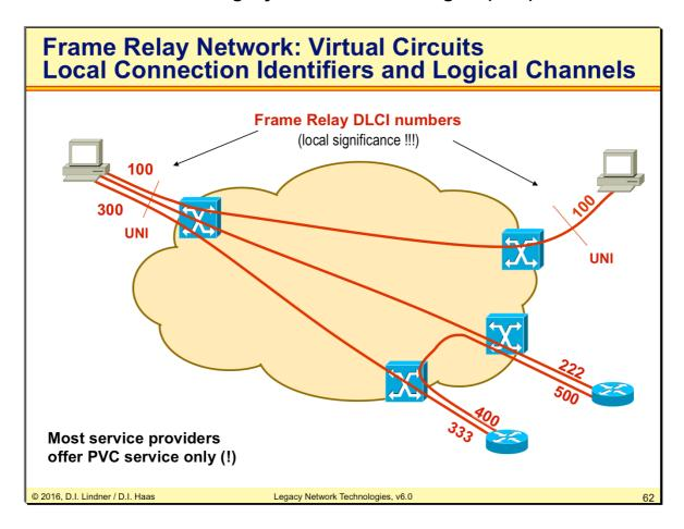
Frame-relay is using virtual circuit identifiers to build up logical channels on one and the same physical Frame-relay connection. The virtual identifiers have local meaning only, that means the must be unique per physical connection only.
