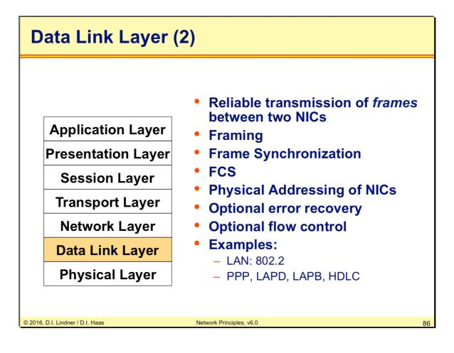
The data link layer builds the frame. In that way, framing or frame synchronization is the most important thing on layer 2. Where is the beginning of the frame ? Where is the end ? With a special Bit-Code the layer 2 protocols, such as HDLC or PPP, guarantee the framing of the data. That's important for the MTU (maximum transfer unit).
