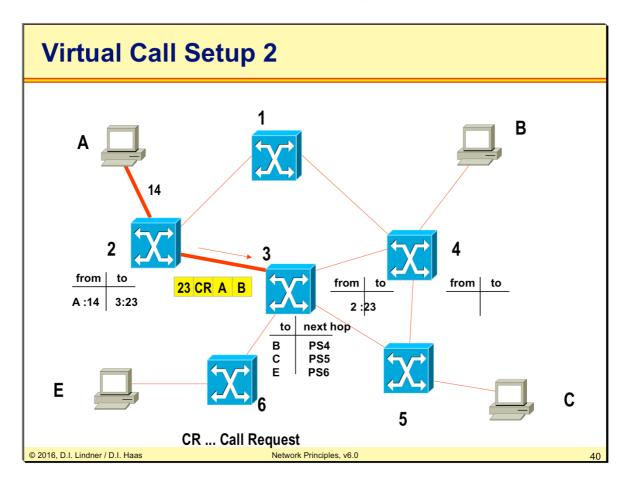
During call setup the information about incoming connection identifier/incoming port to outgoing connection identifier/outgoing port is stored in the **switching table**.
