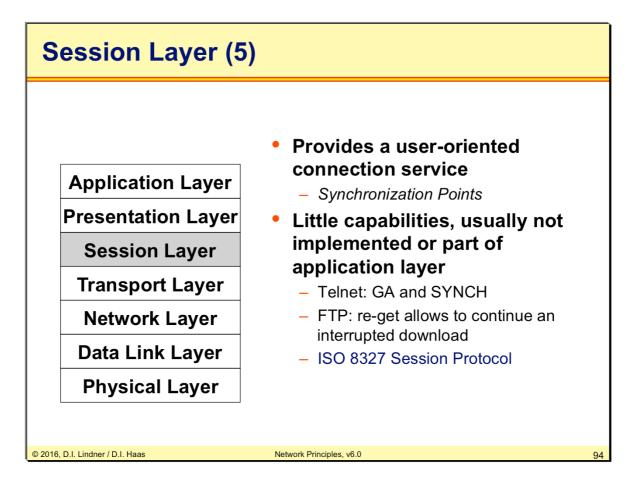
The Session Layer coordinates and controls dialogue between different end systems. This layer is only seldom or sparsely implemented. For example a Telnet server gives the sending permission to the Telnet client via a Go Ahead (GA) sequence. Using the BRK-Key, a SYNCH sequence is triggered and the server must synchronize with the client by flushing the buffered stream. FTP keeps track of the data blocks transmitted and is able to continue an interrupted session from this checkpoint on.
