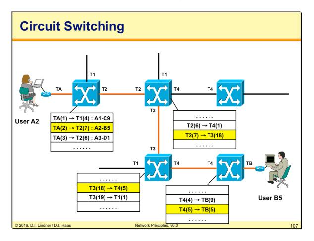
Circuit switching technology is based on deterministic TDM.
