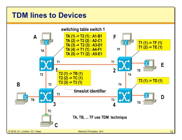
The number of local physical ports can be further reduced by using synchronous TDM between a device and the local switch too. One physical access line may carry many logical channels in corresponding timeslots and hence a mapping between these timeslots can be done in the same way as was already shown for trunk lines.
