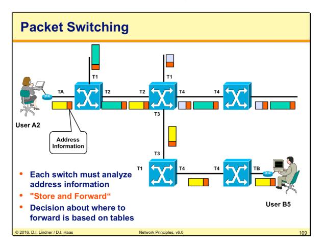
In packet switching technology which is based on statistical time division multiplexing addresses are needed, remember there is no correlation between timeslot and destination. Each switch must analyze the destination address of every data packet to be able to forward it according to some forwarding table.
