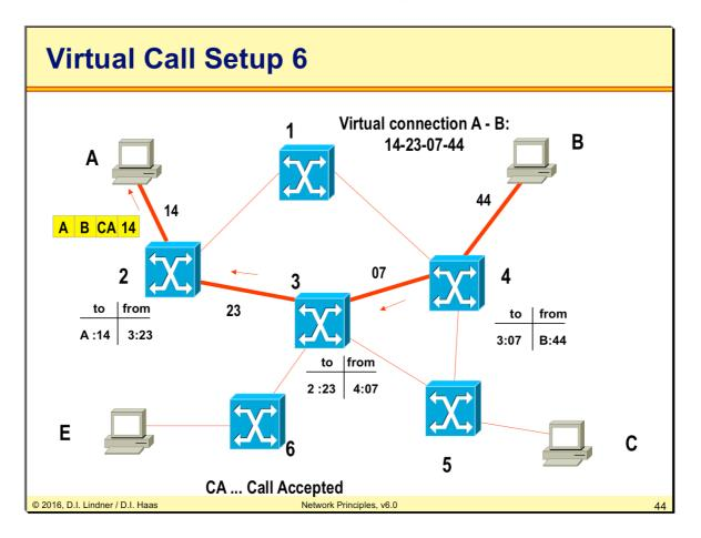
Now the call accepted packet has reached the caller and you can see that the logical point-topoint connection between end system A and B can be identified in the network by the connection identifier sequence 14-23-07-44.
