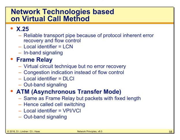
All WAN-switching technologies utilize the same principle that has been described above. But the connection identifier has different names. In X.25 we call it the Logical Channel Number (LCN). With Frame Relay we talk about the Data Link Connection Identifier (DLCI). And ATM packets are switched using the Virtual Path Identifier/Virtual Circuit Identifier (VPI/VCI). No matter what complicated names are used, it is simply a dumb identifier without any special meaning.
