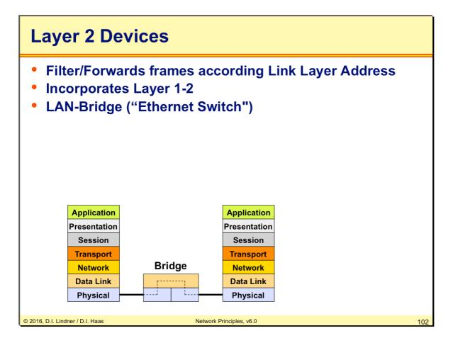
A so called "bridge" or "switch" is a device to connect systems per data link layer. This kind of devices determine the physical layer and can forward datagram's according the link layer address. For example: MAC address with Ethernet. Note that a bridge utilizes two or more physical layer entities (NICs) that is a bridge is able to convert encodings and signal-rates.
