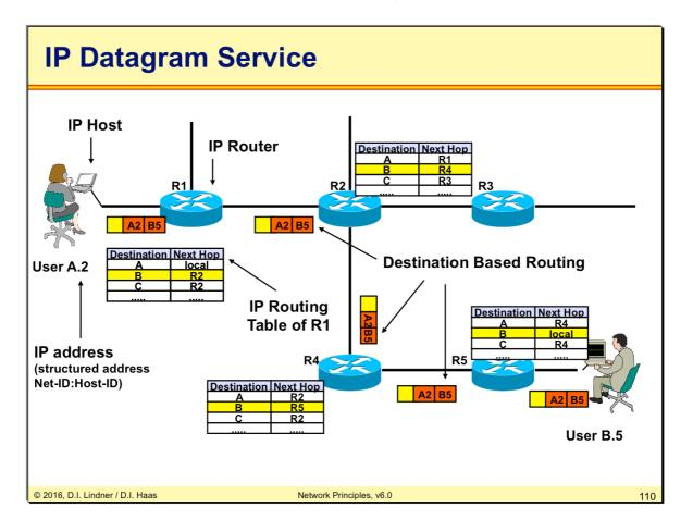
In the Datagram technology user A.2 sends out data packets destined for the user B.5. Each single datagram holds the information about sender and receiver address.
