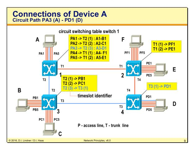
In our example the connection between Port PA3 and PD1 is established by three network switches and their according switching tables. For both users this connection looks like a dedicated point to point link, they are not aware what's going on inside the network cloud.
