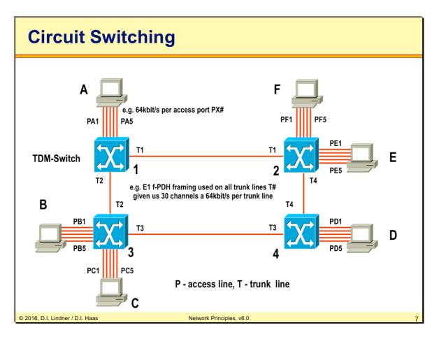
Circuit switching technology is based on synchronous (deterministic) TDM.
