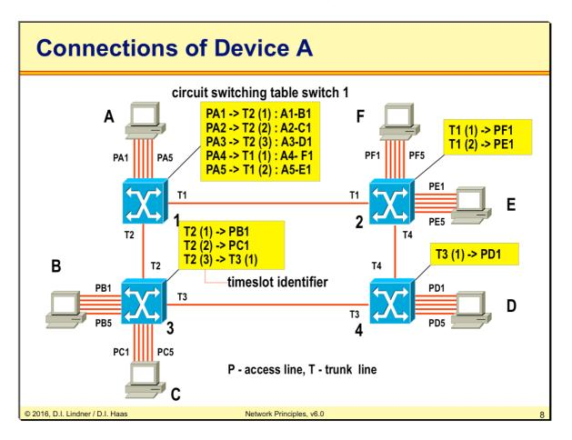
All network switches in circuit switching technology hold a switching table which determines the correlation between
