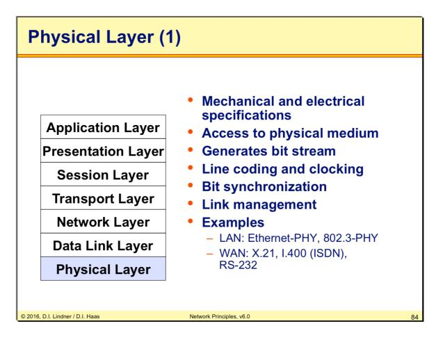
The Physical Layer generates the bit stream. This layer provides access to the physical medium by applying line coding (NRZ, Manchester, etc), bit synchronization (clocking, PLL), but also includes mechanical, electrical and optical specifications. Layer 1 also can activate or deactivate the links between end systems (link management).
