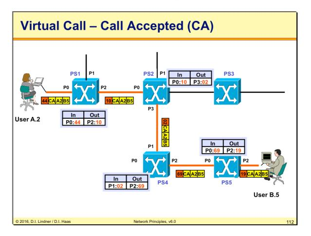
The connection setup request builds up a tunnel-like connection of virtual circuit identifiers held in switching tables.
