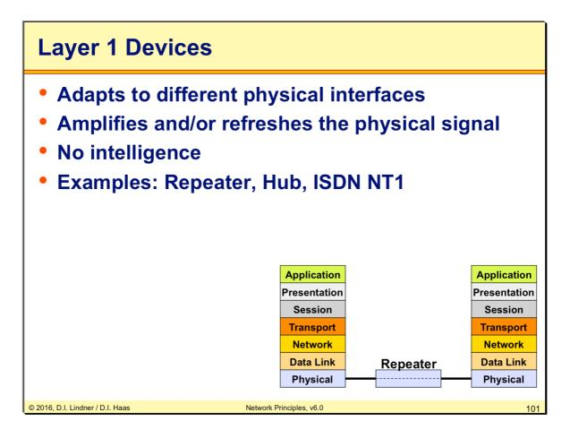
To connect different system with each other we need special devices. If you want to connect two systems only per physical layer you need a so called "hub" or "repeater".
