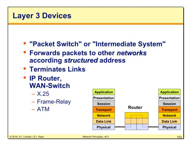
The most important device in the Internet is the so called "router". A router consists of several layer 1 and layer 2 entities and a single layer 3 entity, thus it can forward packets to other networks according structured addresses (remember IP-Addresses). By terminating layer 1 and 2 a router is able to connect total different network technologies with each other. For example: on one side there is Ethernet on the other side ATM.
