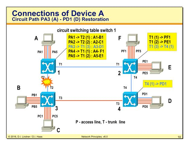
Pictures shows how circuit can be restored by using free timeslots and changed mapping tables along the redundant trunk lines.
