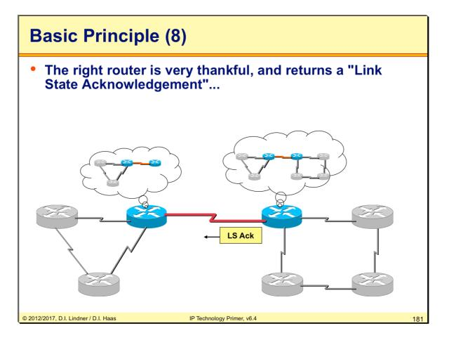
Link State Acknowledgement LSAck is used to make sure that the information is received.
