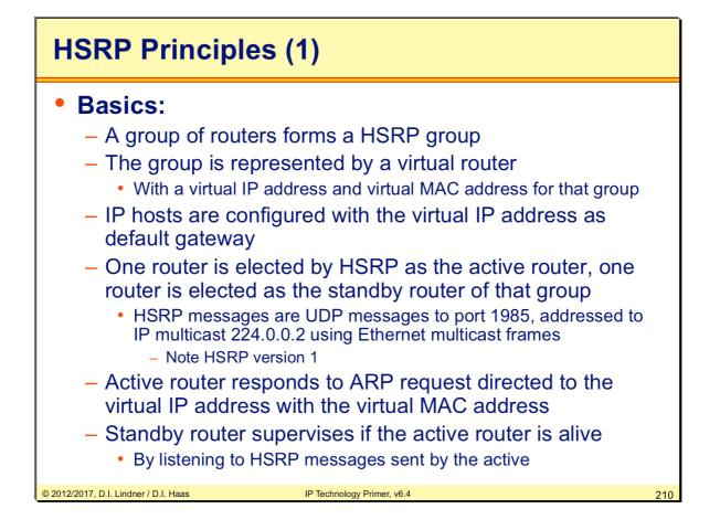
Note: Routers must be able to support more than one unicast MAC address on an Ethernet interface. The active router has to listen to its own MAC address and the MAC address of the virtual router, it represents. That is not the normal behavior of an Ethernet network card. Therefore new network hardware was necessary for routers in order to support HSRP.
