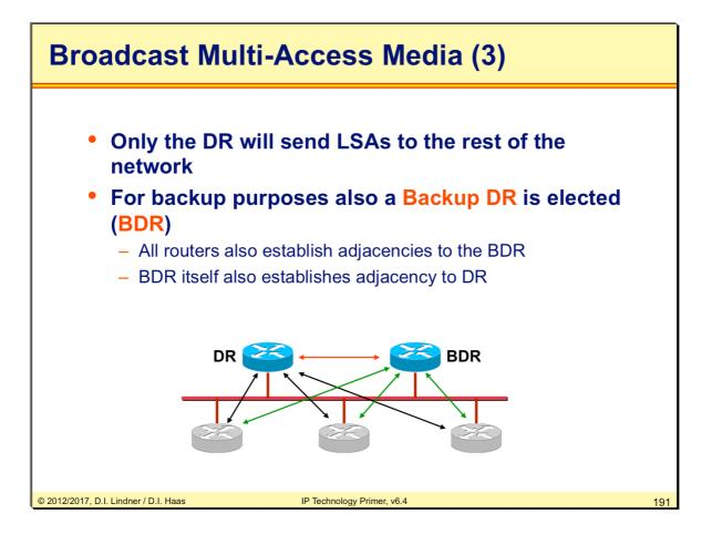
Each multi-access interface has a "Router Priority" ranging from 0 to 255 (default 1). Routers with a priority of 0 cannot become DR or BDR. The election process is performed with Hello packets which carry the priority. If some routers have the same priority, the one with the highest numerical Router ID wins. If a DR fails the BDR becomes active immediately (Hello stays out) and a new election for the BDR is started.
