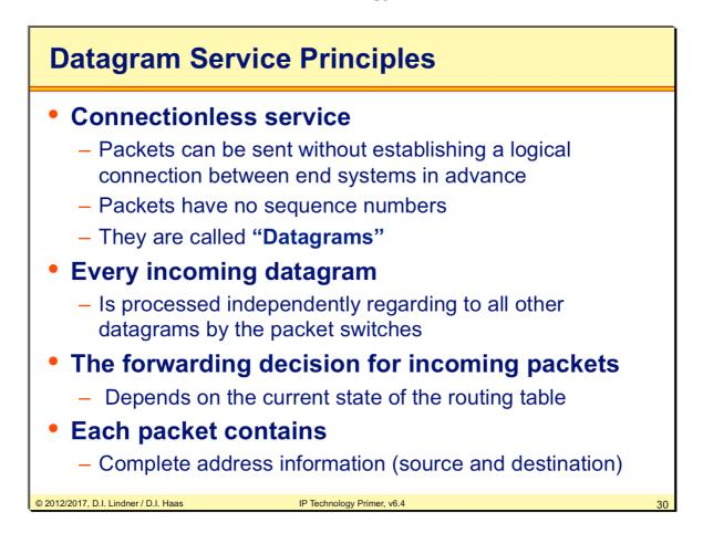
The addresses used in datagram service technologies need to be globally unique and structured. They contain topological information. Structured means a part of the address is reserved for the user identification while another part of the address is used for topology information (describes network where the user is located).
