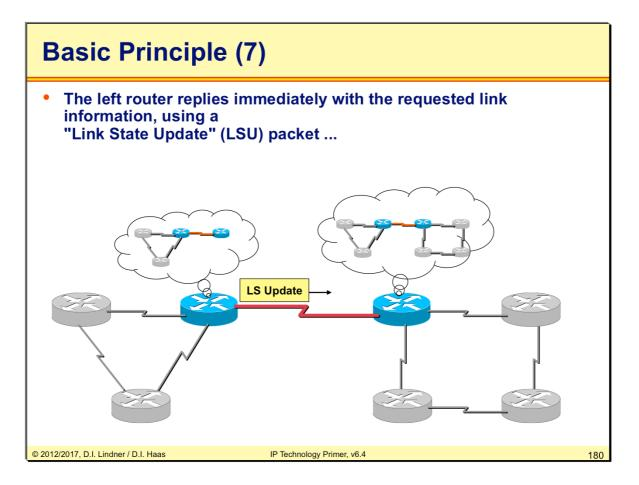
As a reply the left router sends a Link State Update packet LSU which contains detailed information about requested links.
