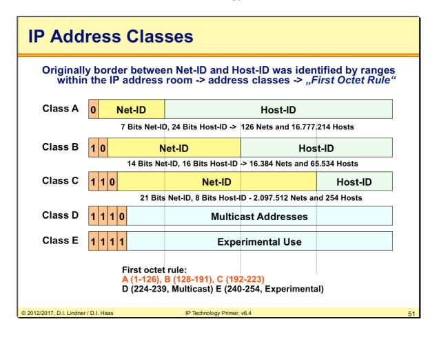
In the beginning of the Internet, five address classes had been defined in order to identity the border between Net-ID and host-ID and a fixed way. The idea of classes helps a router to decide how many bits of a given IP address identify a network number and how many bits are therefore available for host numbering.
