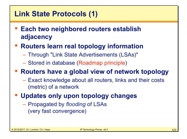
Topology changes (link up or down, link state) are recognized by routers responsible for supervising those links and are flooded by responsible routers to the whole network again by using ( $\underline{L}$ ink  $\underline{S}$ tate  $\underline{A}$ dvertisements, LSAs).
