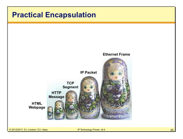
The idea of encapsulation is fundamental in the data communication world. Adjacent layers encapsulate or decapsulate information by adding/removing additional "overheads" or "headers" in order to implement layer-specific functionalities. The whole process can be regarded as Matroschka-puppet principle.
