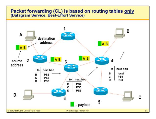
In the datagram technology device A sends out data packets destined for the device B. Each single datagram holds the information about sender and receiver address.
