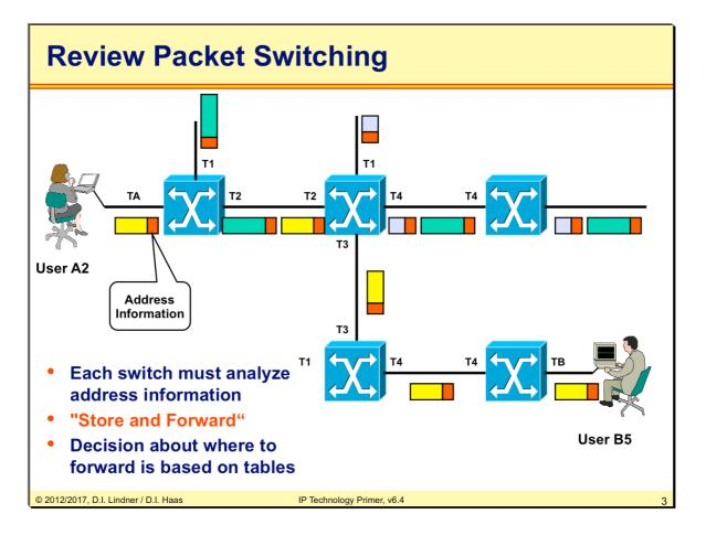
In packet switching technology which is based on statistical time division multiplexing addresses are needed, remember there is no correlation between timeslot and destination. Each switch must analyze the destination address of every data packet to be able to forward it according to some forwarding table.
