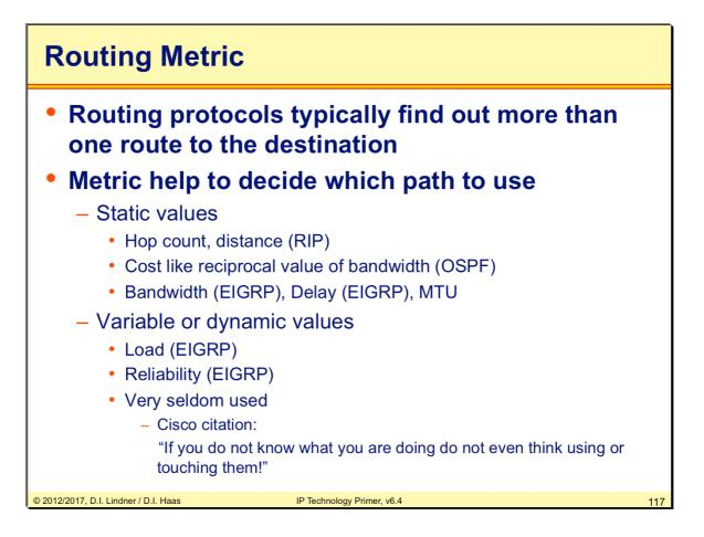
Often router find more than one path to forward a packet to a given destination. The metric helps router find the "best" way. Note that there are several types of metrics used in modern routing protocols. Typically they cannot be compared with each other. For example a simple hop-count is no measure for speed (bandwidth).
