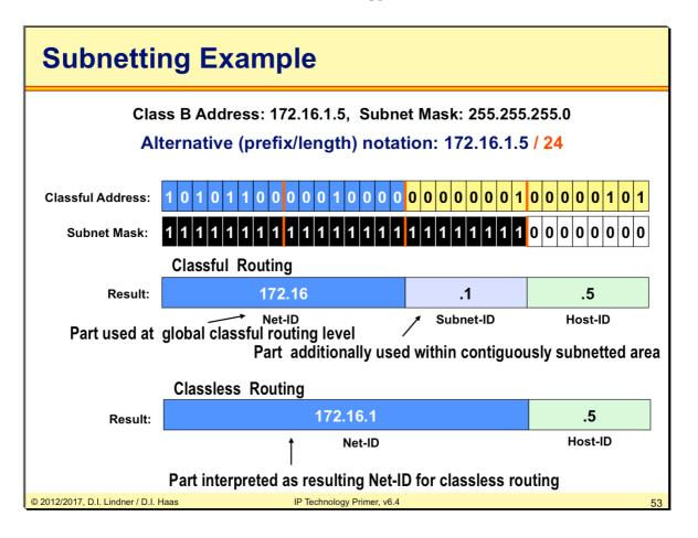
Number of bits to be used for Net-ID and Subnet-ID are specified by subnet mask (also written in dotted decimal notation):
