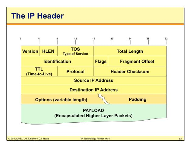
**Version**: Version of the IP protocol. Current version is 4. Useful for testing or for migration to a new version, e.g. IPv6.
