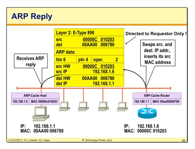
Now station B sees sends an ARP response as a directed MAC frame (SA=Mac\_B, DA=Mac\_A).The ARP response holds MAC address of station B. A stores the MAC- / IP-address mapping for station B in its ARP cache.
