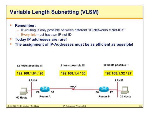
With earlier limitation, an organization is locked into a fixed number of fixed subnets. That is called classful routing. VLSM supports more efficient use of an organization's IP address space. VLSM was created in 1987. RFC 1009 defined how a subnetted network could use more than one subnet mask.
