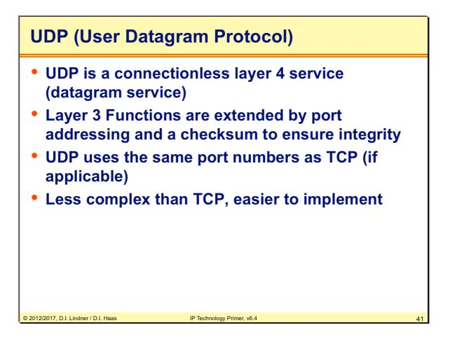
UDP is connectionless and supports no error recovery or flow control. Therefore an UDP-stack is extremely lightweight compared to TCP.
