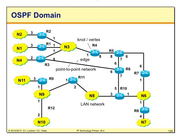
With this topology-database a router can calculate the best path to all destination-networks by applying Dijkstra's SPF (Shortest Path First) algorithms.
