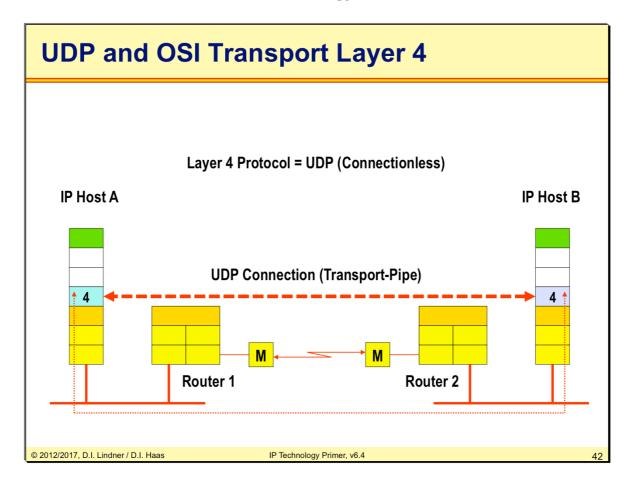
Recognizes that even the IP hosts see a transport pipe, this pipe is unreliable.
