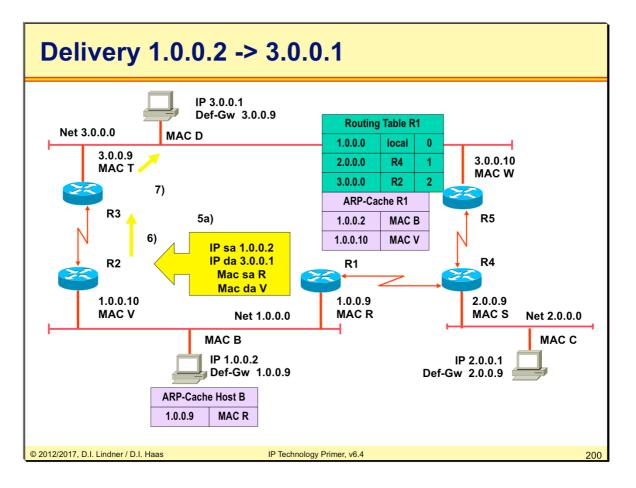
At router R1 the IP datagram is forwarded on the same interface as it was received -> redirect would be nice to avoid sending this datagram twice on net 1.0.0.0.
