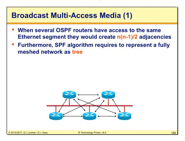
Basic concept of link state requires point-to-point relationships. That fits best for point-to-point networks like serial lines but that causes a problem with shared media multi-access networks (e.g. LANs or with networks running in a so called NBMA-mode (Non Broadcast Multi Access) like X.25, Frame Relay, ATM. Hello, database description and LSA updates between each of these routers can cause huge network traffic and CPU load.
