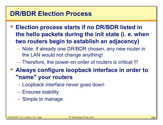
It is recommended in OSPF to use the loopback interfaces for router ID. You should configure a loopback interface first and then start the OSPF process, otherwise the highest ip address from a physical interface will be taken.
