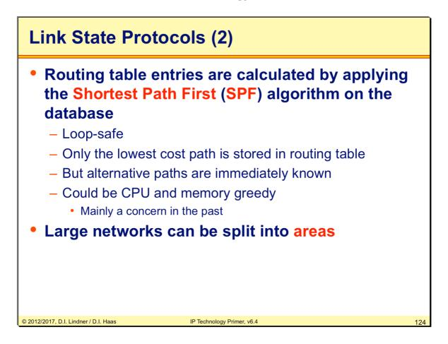
Applying the SPF algorithm on the link state database, each router can create routing table entries by its own.
