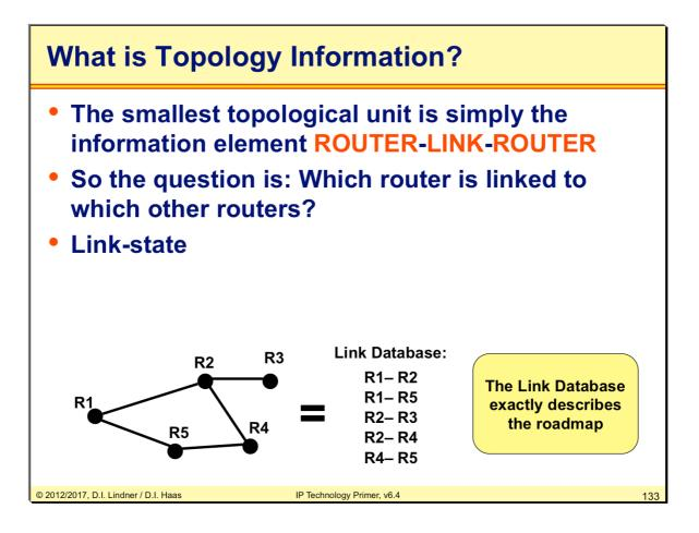
Obviously the dots are routers and the links between the routers are actually networks. The basic idea of OSPF and the topology table is that simple.
