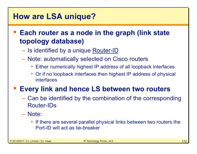
Note that loopback interfaces are more stable than any physical interface. Furthermore it's easier for an administrator to manage the network using loopback addresses for Router-IDs.
