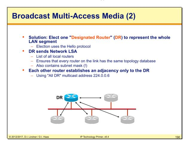
To prevent the problems described in the previous slide, a Designated Router (DR) is elected on a multi-access network. DR is responsible for representation of the multi-access network and all the routers on it to the rest of network and management of flooding process on a multiaccess network. The network itself becomes a "pseudonode" on the graph. The pseudonode is represented by the DR.
