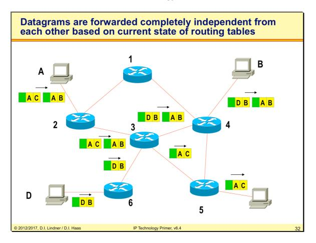
The routing tables can be set up either by manual configuration of the administrator or by the help of dynamic routing protocols ( in case of IP that are protocols like RIP, OSPF, IS-IS, etc). The use of dynamic routing protocols may lead to rerouting decisions in case of network failure and so packet overtaking may happen in these systems.
