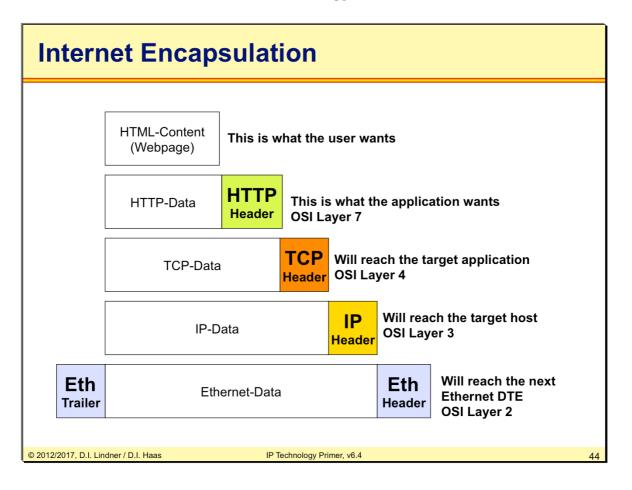
In our example let's suppose a webserver sends a webpage (HTML code) to a client. The webpage is carried via the Hyper Text Transfer Protocol (HTTP) which provides for error and status messages, encoding styles and other things. The HTTP header and body is carried via TCP segments, which are sent via IP packets. On some links in-between, the IP packets might be carried inside Ethernet frames.
