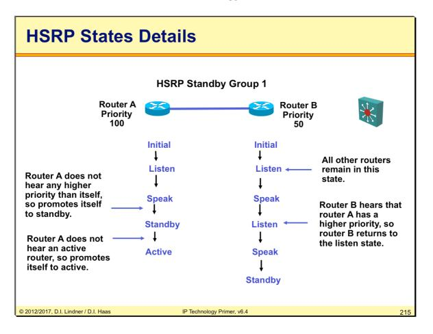
*Initial state*— All routers begin in the initial state. This state is entered via a configuration change or when an interface is initiated.
