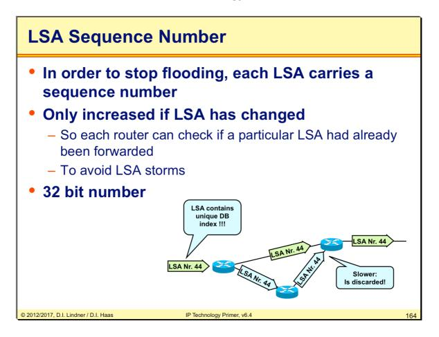
When reaching the end of the 32 bit sequence number the associated router will wait for an hour so that this LSA ages out in each link state database. Then the router resets the sequence number (lowest negative number i. e. MSB=1, 8000001) and continues to flood this LSA.
