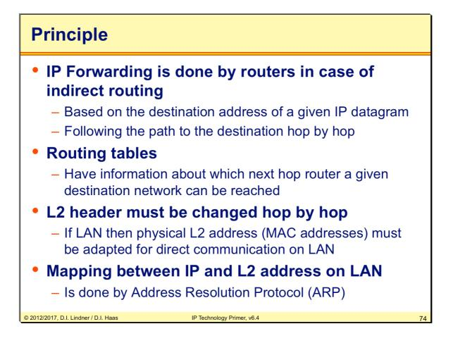
Note that also simple workstations and PCs maintain routing tables—but not for routing passthrough packets, rather locally originated datagrams should be routed to the most reasonable next hop. Typically, the routing table consists only of a single entry, which is the default gateway for this host. But also additional entries can be made, indicating other gateways for some dedicated routes.
