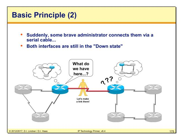
After the link is connected, the routers detect a new network (OSPF is configured on the interface and interfaces are enabled).
