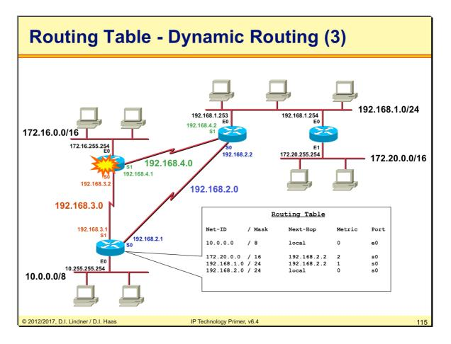
In our example loss of left router causes adaption of the routing table networks 172.16.0.0, 192.168.3.0 and 192.168.4.0 are not longer seen in the routing table If left router comes back the dynamic routing will learn about these network again, hence we can see the automatic appearance of networks in a routing table in case of power on.
