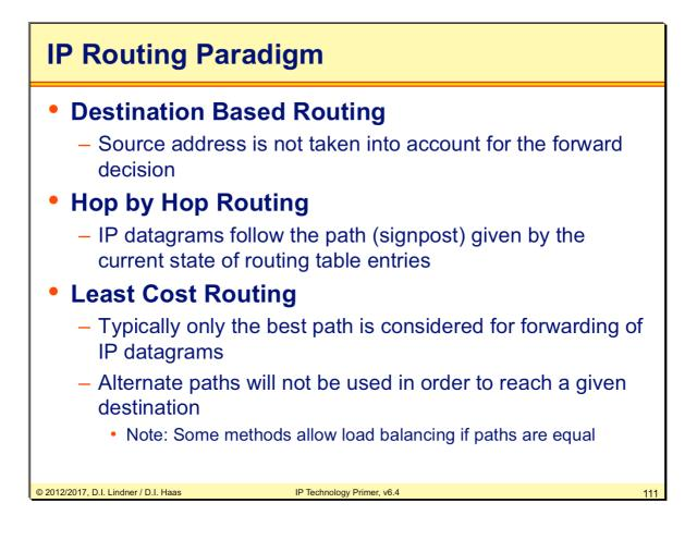
The IP routing paradigm is fundamental in IP routing. Firstly, IP routing is "destination based routing", that means the source IP address is never examined during the routing process. Secondly, IP routing is "hop-by-hop", which emphasizes the difference to virtual circuit principles. The routing table in every router within the autonomous system must be both accurate and up to date (consistent and loop-free) so that datagrams can be directed across the network to their destination.
