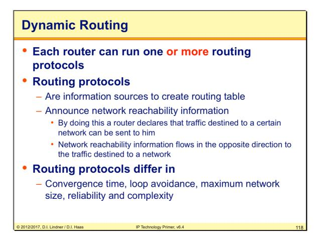
In contrast to static routing where every route must be configured manually, dynamic routing works with one or more routing protocols. These protocols inform the router and create the routing table automatically. Widely used in the Internet. Convergence time is the time until all routers will have the same consistent view of the network after a topology change. Until that temporary routing loops are possible, if entries in routing tables point to each other or lead to circles.
