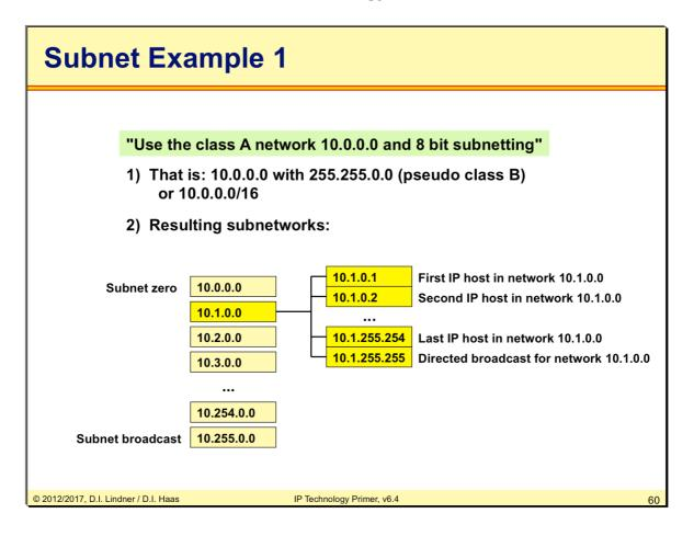
The example above shows how to subnet a class A network—in our case network 10. Here we use a 16-bit subnet mask allowing us to define  $2^8 - 2$  subnets, because the natural subnet mask of a class A network is 8 bits in length.
