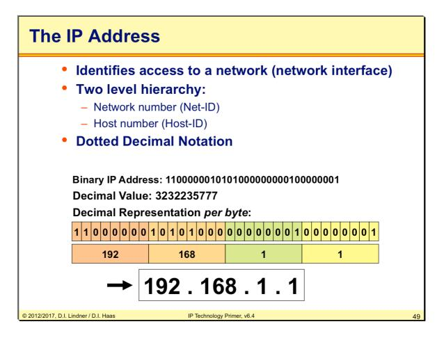
The IP Address is a 32 bit value in the IP header. The address identifies the access to a network. Always keep in mind that IP addresses are basically simple numbers only. There is no natural structure in it.
