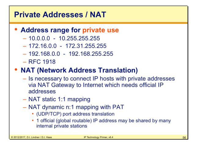
So-called RFC 1918 addresses are class A, B, and C address blocks which can be used for internal purposes. Such addresses must not be used in the Internet. All gateways connected to the Internet should filter packets that contain these private addresses. Furthermore these addresses must not be used in Internet routing updates.
