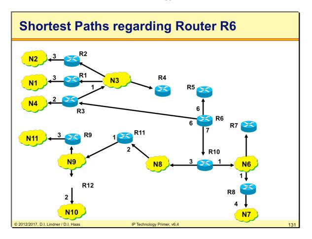
After calculating the shortest path the routing table is constructed by just adding next hop and summary metric taken from the shortest path tree for every network.
