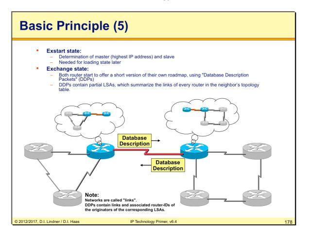
After neighborship is established, the routers enter the "exstart state" and determine who of them is master and who is slave. This will be needed later as the master will begin to send LS-Request packets. The rule is simple: the router with the highest IP address (of the two involved interfaces on that link) is master.
