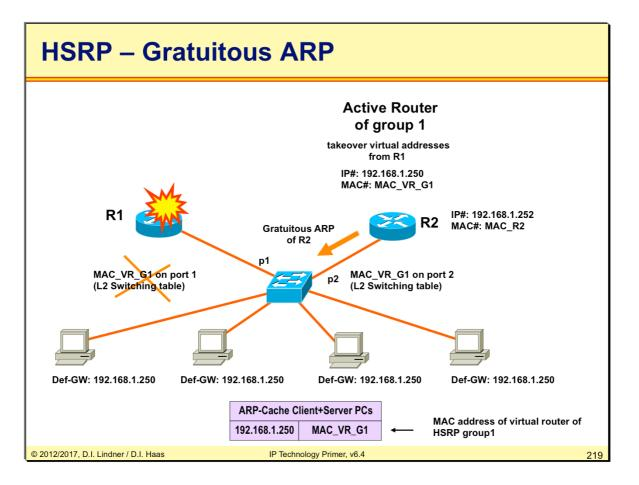
Gratuitous ARP has to be sent by router R2 in order to actualize the MAC address table of the underlying L2 Ethernet switches. Now port p2 points to the virtual Mac address MAC\_VR\_G1.
