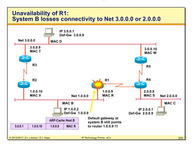
Imagine what happens when R1 is lost. IP host 1.0.0.2 can nor reach any foreign IP network anymore, because it still points to MAC R of 1.0.0.9. We have a black-hole problem. Even after ARP cache times out there is still no automatic possibility for IP host 1.0.0.2 to switch to router R2.
