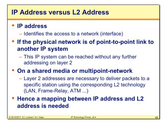
On a multipoint network every station needs a layer-2 address. When IP packets should be sent to a local destination the sender must first determine the corresponding layer-2 address. A multipoint network is also known as a shared medium. It could be a broadcast domain (like Ethernet) or not (like Frame-Relay or ATM). Therefore the layer-2 address could be a MAC address, a DLCI (Frame-Relay) or similar. In this chapter we only focus on Ethernet only.
