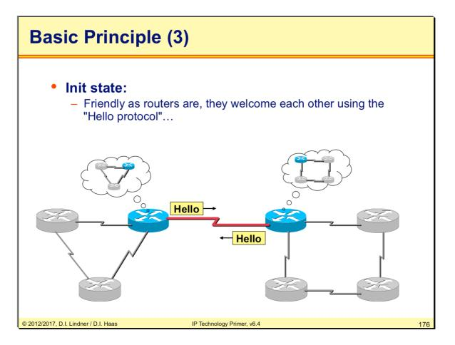
OSPF routers send Hello packets out all OSPF enabled interfaces on a multicast address 224.0.0.5. Then the router waits for a reply (another hello from the other side) which must arrive within 4 x hello interval, otherwise the router falls back to the down state again. That is, the init state lasts only up to 4 times the hello interval.
