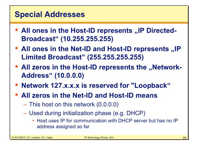
A network broadcast is used to send a broadcast packet to a dedicated network. The IETF strongly discourages the use of IP directed broadcast and it is not defined for IPv6.
