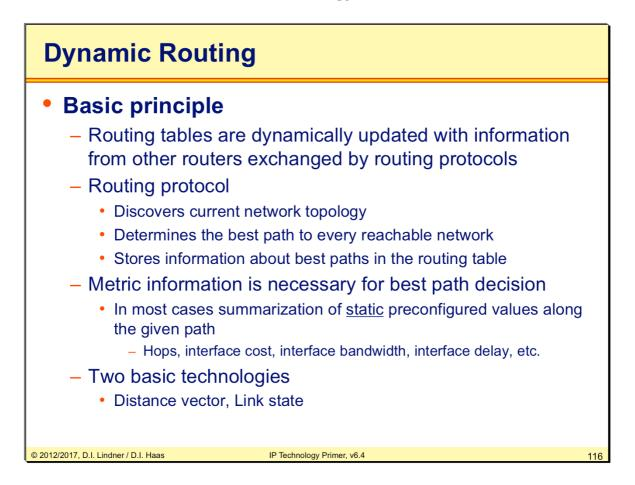
What can a dynamic routing protocol detect? Basically only loss of links and loss of routers. In case of redundancy an alternate route will be stored in the routing table.
